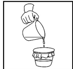
**Choose a disinfection method.** Boiling and chemical treatment are two general methods used to effectively disinfect small quantities of filtered and settled water.
