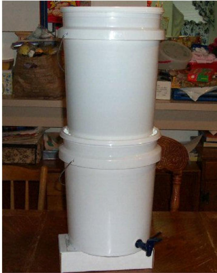
To use the filter, fill the upper bucket with water and wait. If you are starting with dry elements, it will take quite a while before the water starts dripping into the lower bucket. It takes up to several hours for the clean water to drain into the lower bucket. This process can be sped up considerably by frequently topping off the water in the upper bucket. This maintains maximum pressure on the elements.
