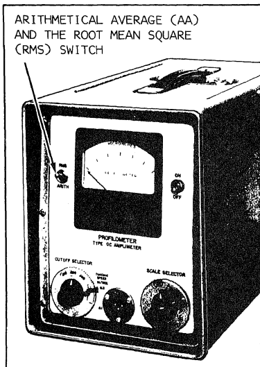
Figure 3-11.—The profilometer amplimeter control panel.
