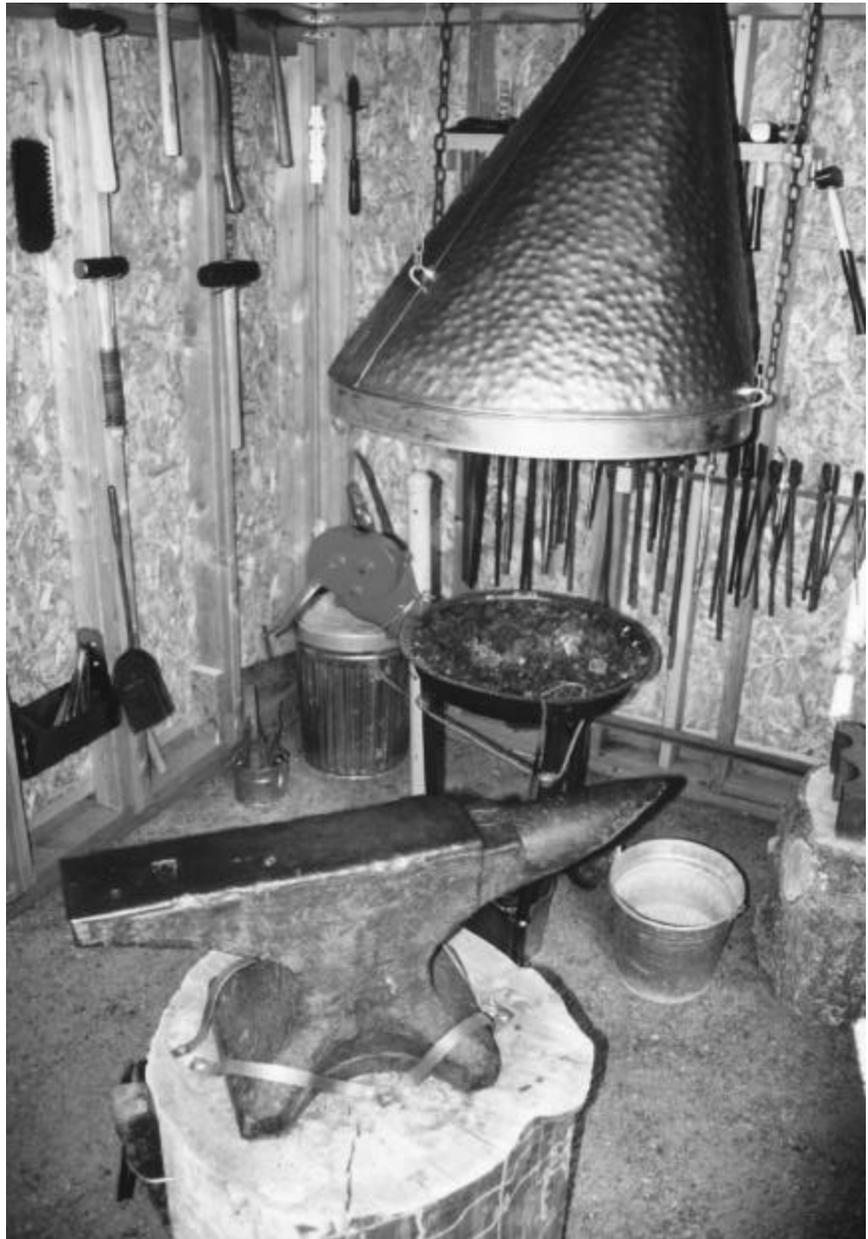
*An anvil and forge can be especially handy for making and repairing other tools.*
