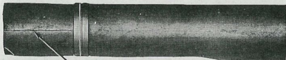
DAMAGED AND WILL EFFECT STRENGTH. THIS GUARD IS NOT ACCEPTABLE.
