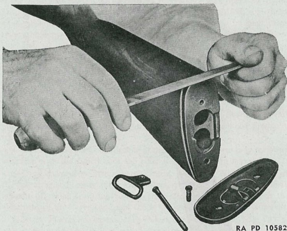
Figure 74. Fitting butt plate on stock.
