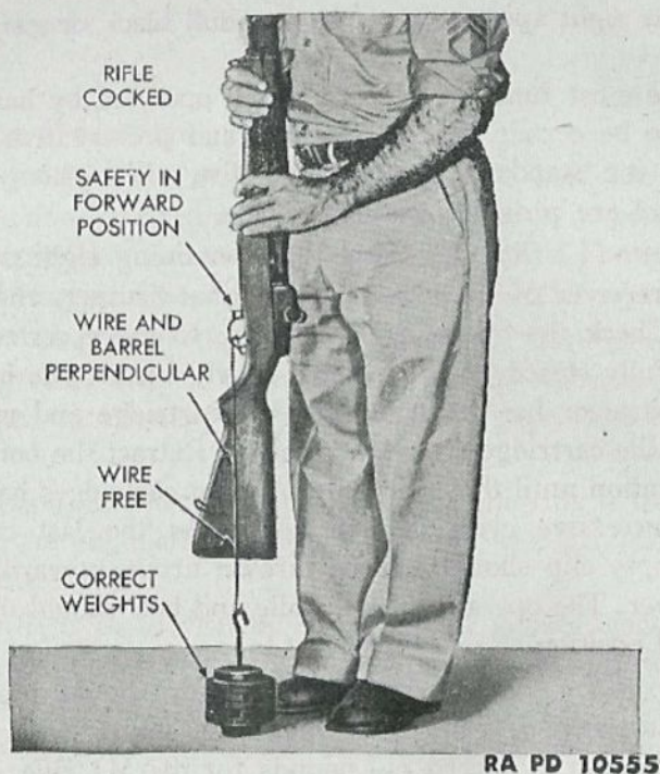
Figure 4. Checking trigger pull with weights.
