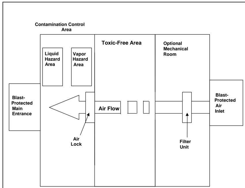
Figure VII-1. General Layout for an NBC Shelter
