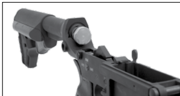
FIG 38 BUFFER AND RECOIL SPRING REMOVAL
