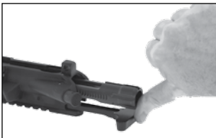
FIG 47 REINSTALLATION OF THE BOLT CARRIER ASSEMBLY TO UPPER RECEIVER
