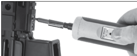
FIG 52 TIGHTENING OF RAIL CLAMP SCREWS
