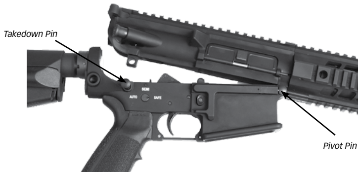
FIG 27 THE TAKEDOWN PIN AND PIVOT PIN
