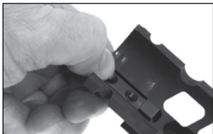
FIG 48 QUAD KEY AND RAIL CLAMP PRE-ASSEMBLED
