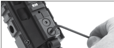
FIG 32 REMOVAL OF CLAMP SCREWS AND CLAMP
