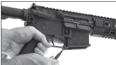
FIG 16 TRIGGER AND GUARD RELEASE
