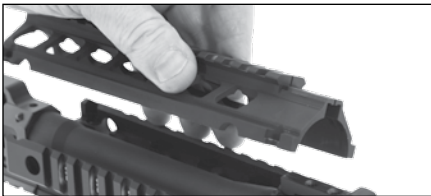
FIG 50 RE-INSTALLATION OF LOWER RAIL SECTION
