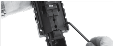
FIG 51 TIGHTENING OF RAIL SECTION SCREWS
