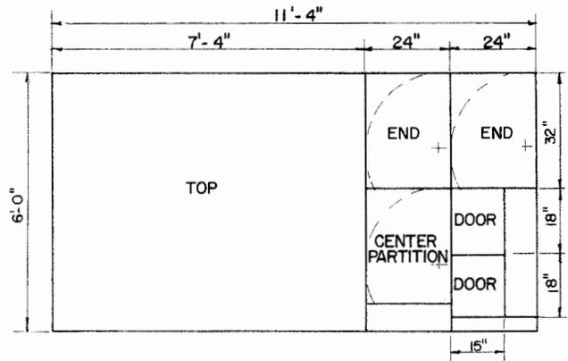
**WIRE MESH CUTTING DIAGRAM**
