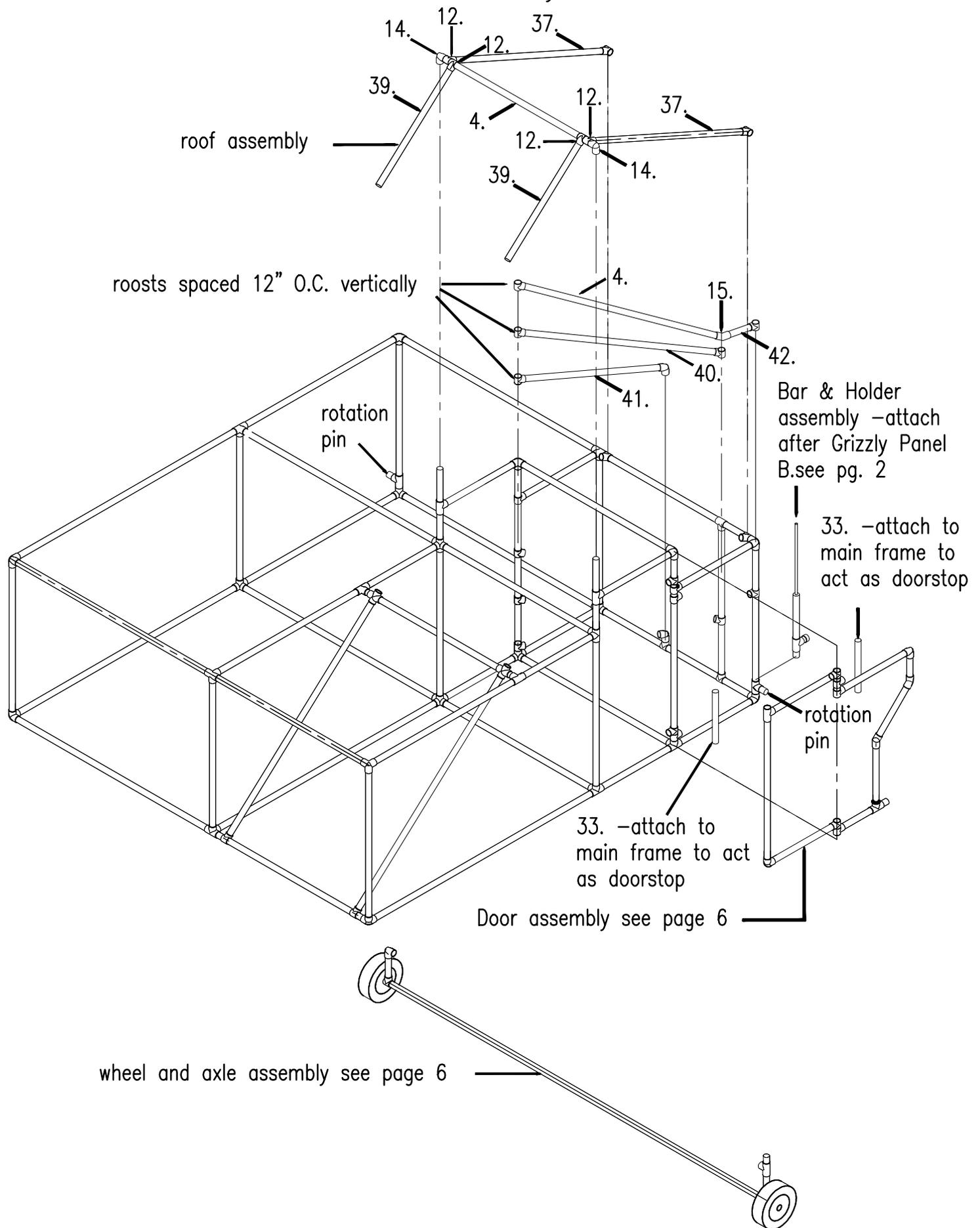
Wheel & Axle assembly rotates about rotation pins. Wheels & Axle shown shaded in the up position
