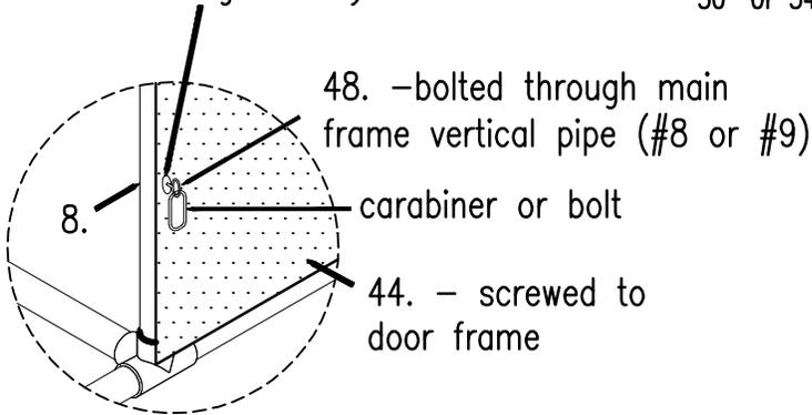
48. - bolted through main frame vertical pipe (#8 or #9)
