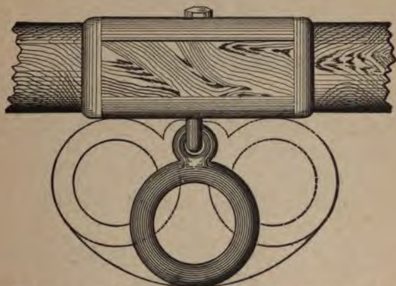
Making a Staple and Ring for a Neck Yoke by the Method of "M. D. D." Fig. 32—The Finished Ring.
