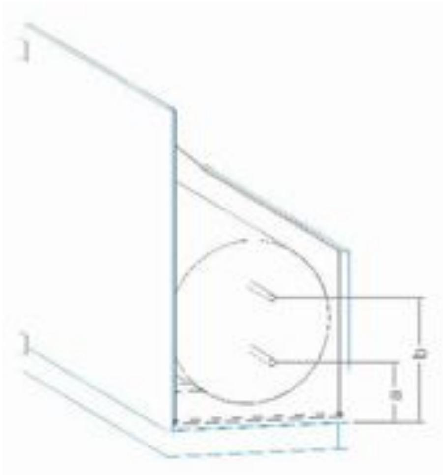
14. Place the unattached "Side" wall and insulation down on the ground. Find the horizontal center of the "Side" wall along the bottom edge. From this point, vertically measure and mark the two vertical distances for the inlet holes.
