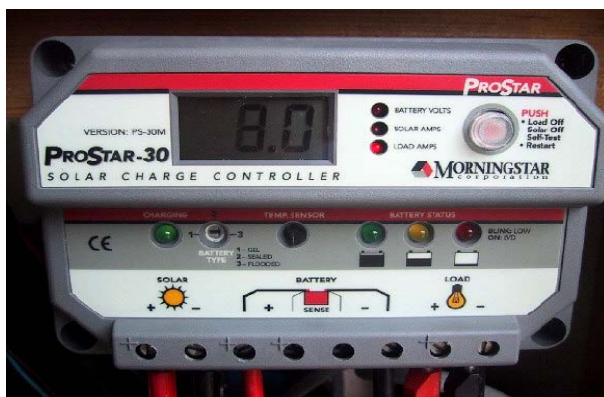
A charge controller showing the voltage in a battery bank.
