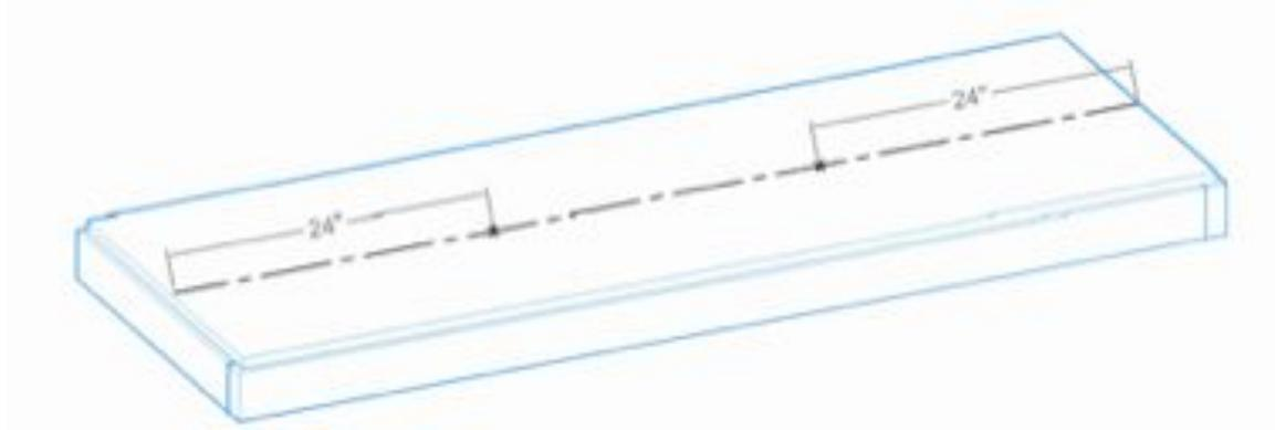
Note: To aid in placing the tank braces, measure 1 1/4" off of each side of the mark. Use a carpenter or speed square to mark the position of the braces on the bottom plywood sheet as shown.
