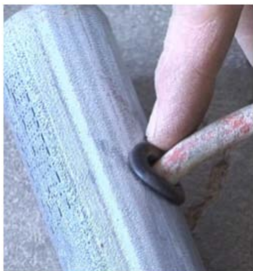
Hole with rubber grommet installed at bottom
