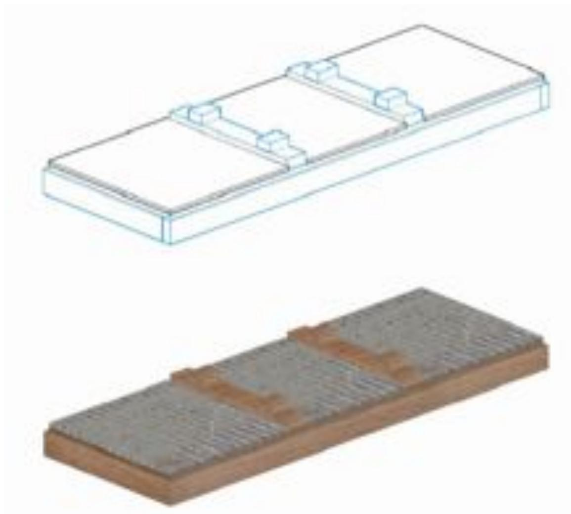
11. Attach insulation pieces #4, #5, #6, and #7 to the walls of the batch collector. Be sure they are aligned correctly. See sketch.
