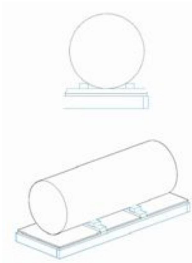
10. Remove the water tank from the brace pieces. Attach the 2 1/2" pieces to the 24" pieces according to the place markings you made in step 9.
