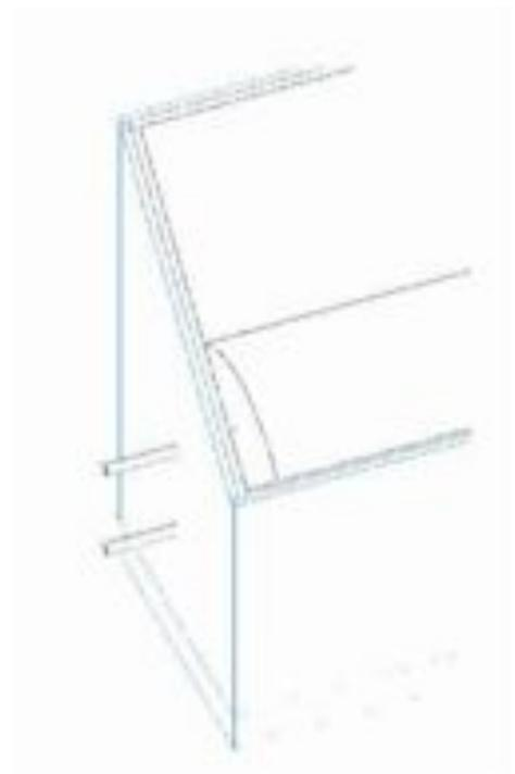
17. Seal "Side" wall insulation joints with reflective tap.
