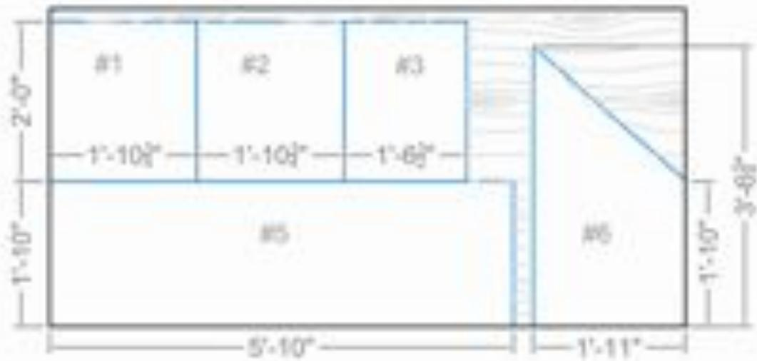
8. Attach insulation pieces #1, #2, and #3 to the "Bottom" plywood piece between the tank braces.
