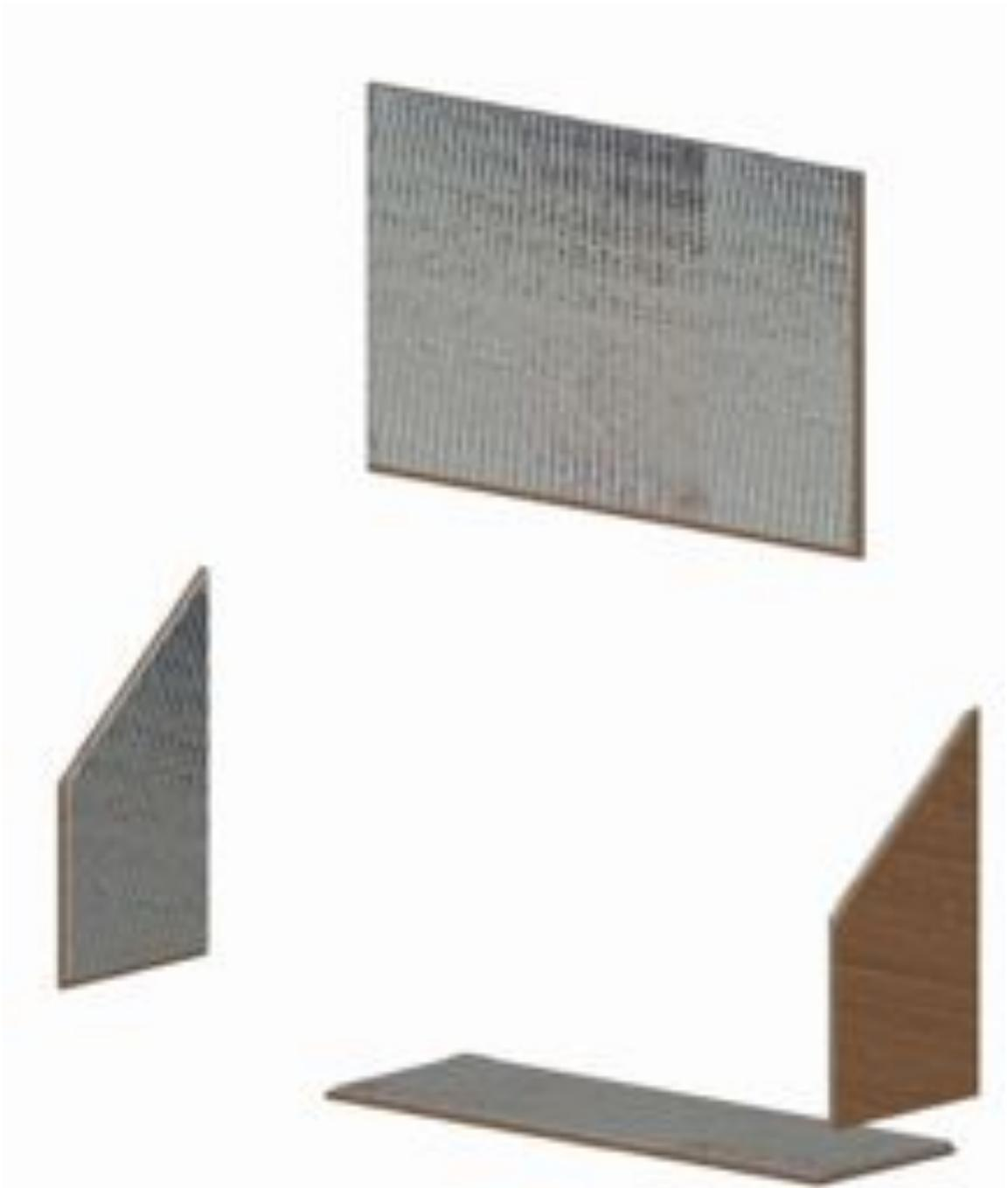
Assemble batch collector box. Attach "Front" and "Back" walls first. Then add only one "Side" wall. Leave the final "Side" wall for later. Use wood-to-wood connectors on exterior corners. Everything should fit together tightly.
