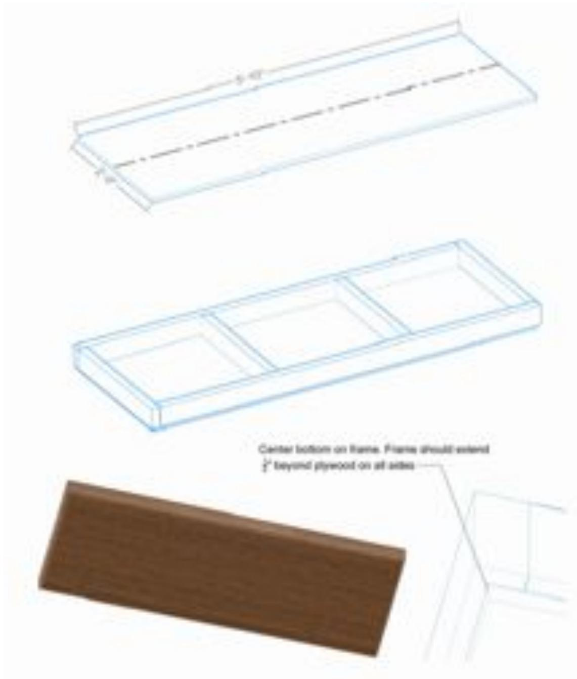
5. Starting at either of the short ends of the "Bottom" plywood piece, measure 24" along the centerline toward the center of the piece. Mark this spot. Do the same measurement and marking from the opposite end.
