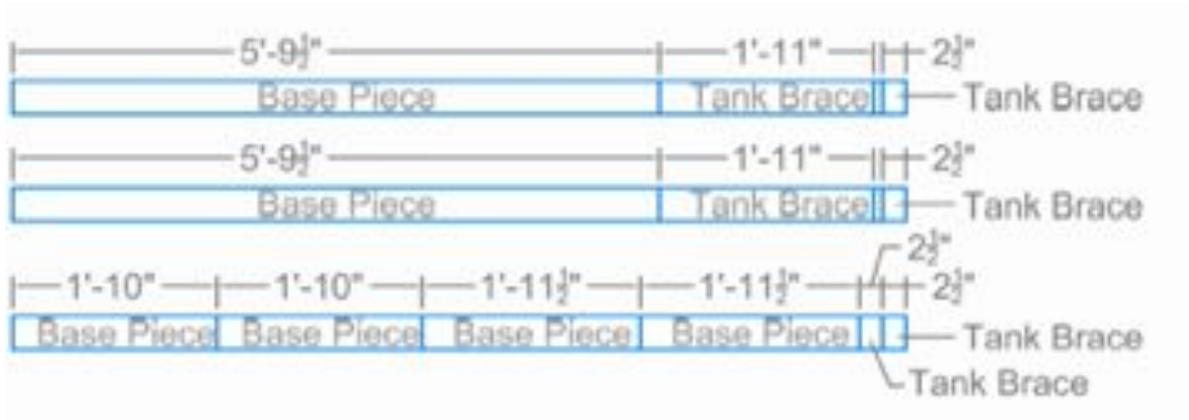
2. Assemble base using 3" lag screws. Keep in mind that the actual dimension of "2 in. x 4 in." lumber is 1.5 in. x 3.5 in.
