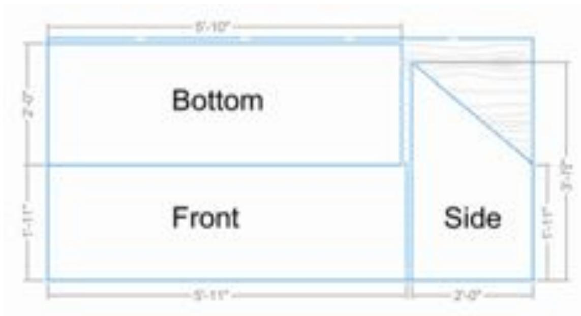
4. Find the "Bottom" plywood piece. Draw a centerline down the length of the piece. Attach the plywood piece to the 2" x 4" lumber base with lag screws. Make sure the plywood piece is centered on the base. The base should extend 1/2" beyond the plywood on each side. See sketch below.
