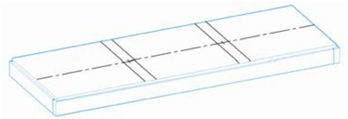
6. Attach the large brace pieces. Start by marking the center of the two 24" pieces of the tank braces. Align the center markings on the two 24" pieces with the two markings on the centerline of the "Bottom" plywood piece. Using 3" lag screws, attach the two 24" tank brace pieces to the "Bottom" piece as shown in sketch. Keep track of remain 2 1/2" tank brace piece from step 1.
