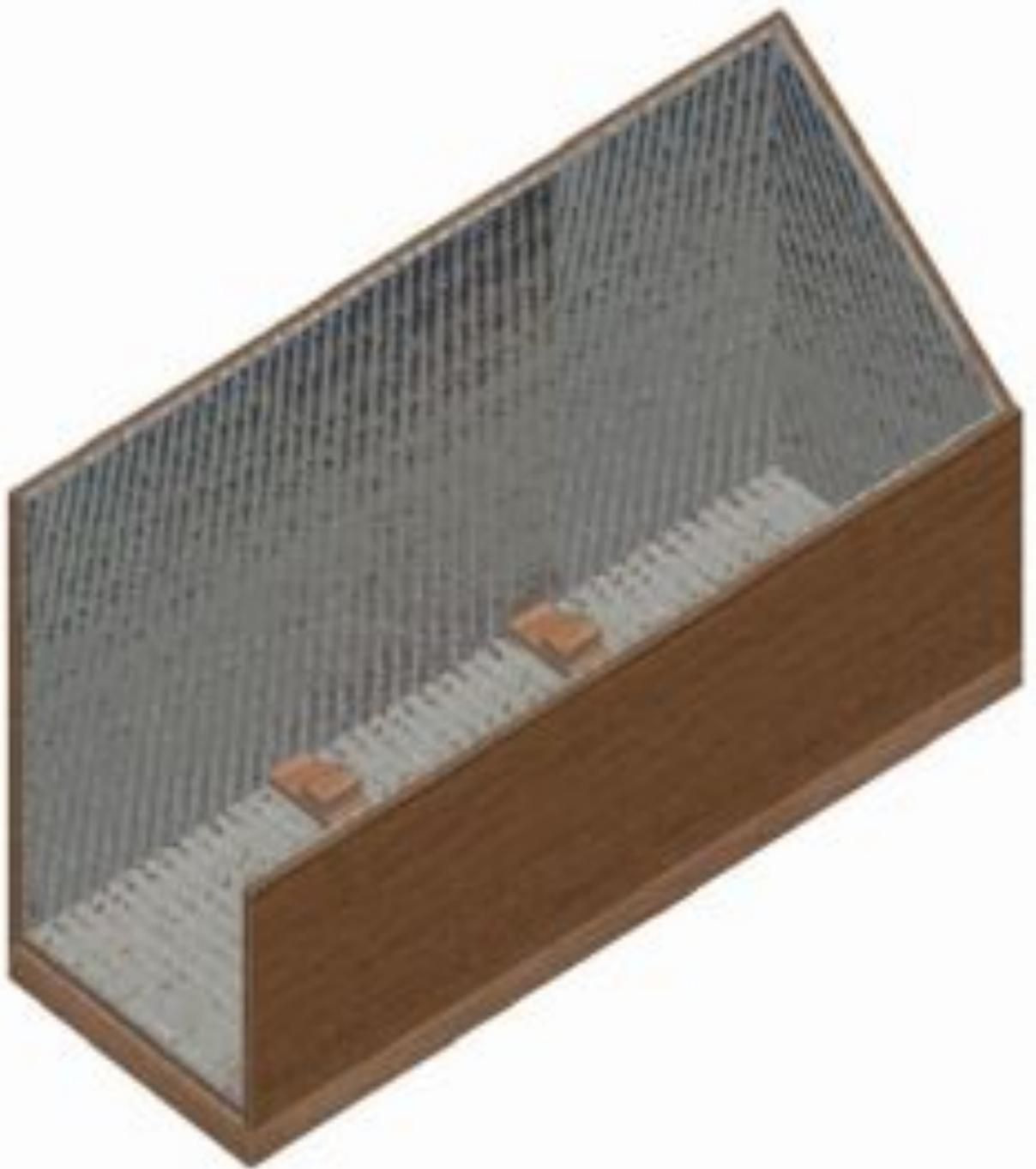
12. Seal insulation joints inside the collector with 2" reflective tape.
