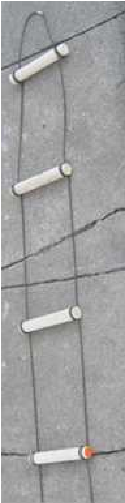
Paracord is strong enough to make a simple rope ladder, using sticks or lengths of dowel. Braid three cords together, if you need a stronger ladder.
