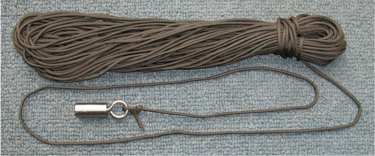
A small weight and a length of paracord make a handy throwing line.
