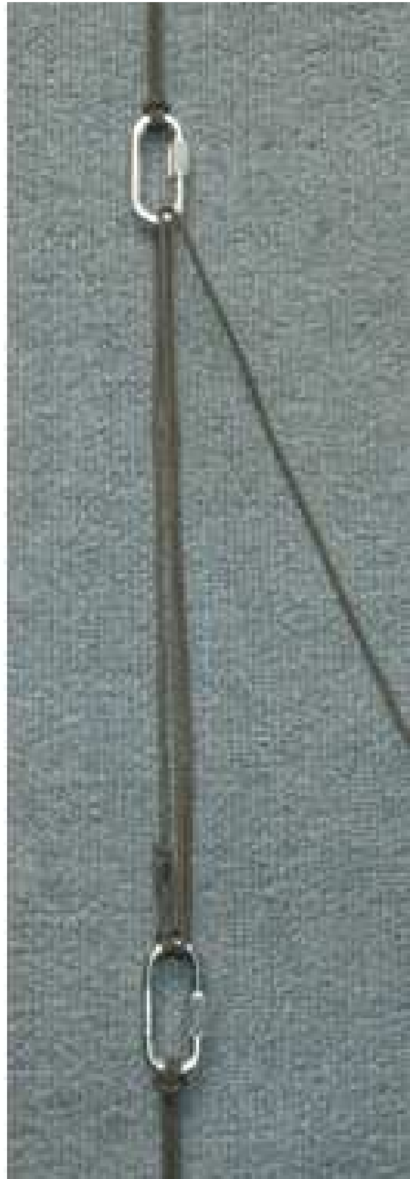
Paracord can be looped through two chain repair links, or two carabiners, to make an improvised hoist.
