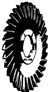
Figure 11-28.—Slitting saw with side teeth.
