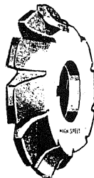
Figure 11-42.—Corner rounding cutter.
