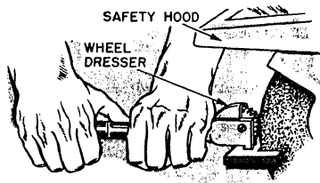
Figure 6-9.—Using a grinding wheel dresser.
