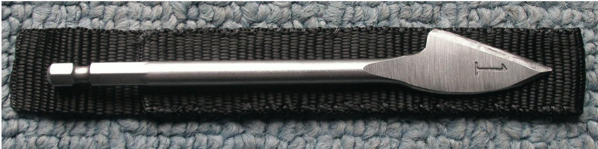
This is the Hoffman harpoon, which I made from a one-inch spade-style wood-boring drill bit.
