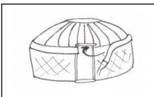
Tie the end of the canvas tension band to the frame, inside of the door. Pass it around the outside of the yurt, where the roof and walls meet. Pull it tight as you go, but not so tight that it lifts the roof. Tie the other end securely to the frame inside of the door.
