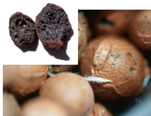
Close-up view of young tomato root as it grows into expanded clay aggregate. Inset shows inner porosity of LECA stone.
