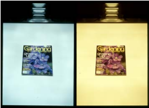
On the left is a Metal Halide lamp, notice the white/blue hue. The lamp on the right is a High Pressure Sodium and exhibits a warmer, yellow/orange hue.
