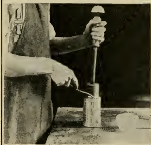
FIG. 57. Capping and Tipping a Solder Top Can. (1) Wipe off groove and cap with cloth to remove sirup, pulp, etc.; (2) Wipe groove with brush dipped in soldering fluid; (3) Apply hot capping steel and melt solder of solder hemmed cap or melt a little solder from solder wire; (4) Turn the steel two or three turns backward and forward to distribute solder evenly; (5) Raise the steel, but hold lid down for 2 or 3 seconds by center rod to allow solder to set; (6) wipe vent hole with soldering fluid; apply hot tipping steel and seal with drop of solder.
