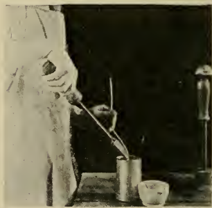
FIG. 57. Capping and Tipping a Solder Top Can. (1) Wipe off groove and cap with cloth to remove sirup, pulp, etc.; (2) Wipe groove with brush dipped in soldering fluid; (3) Apply hot capping steel and melt solder of solder hemmed cap or melt a little solder from solder wire; (4) Turn the steel two or three turns backward and forward to distribute solder evenly; (5) Raise the steel, but hold lid down for 2 or 3 seconds by center rod to allow solder to set; (6) wipe vent hole with soldering fluid; apply hot tipping steel and seal with drop of solder.
