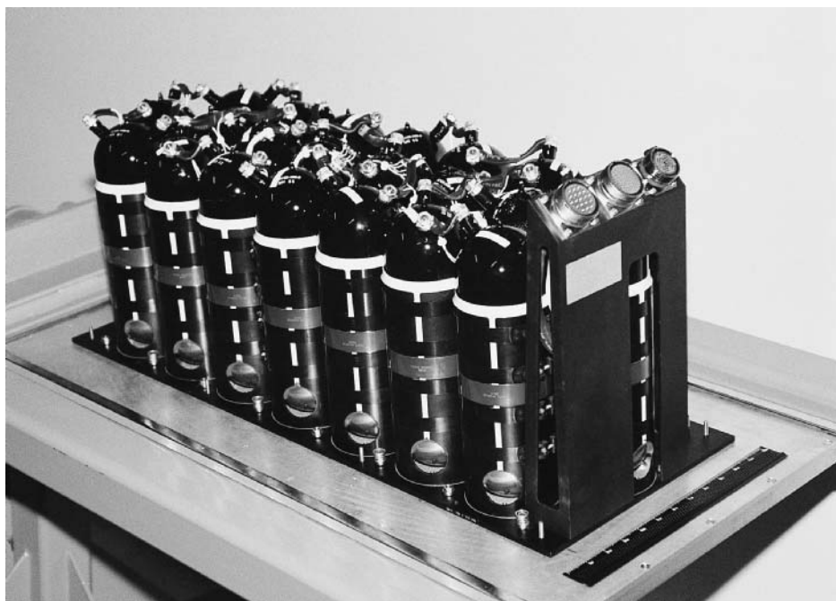
FIGURE 32.6 DMPS 100-Ah Ni-H 2 battery assembly.
