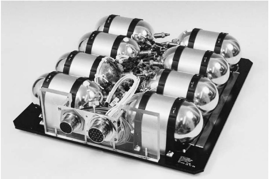
FIGURE 32.24 Mars Global Surveyor 23-Ah CPV battery assembly.
