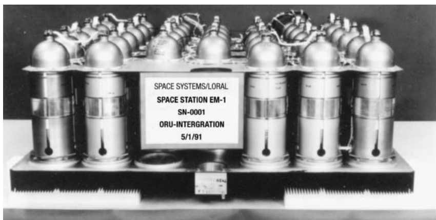
FIGURE 32.8 International Space Station 81-Ah Ni-H 2 38-cell assembly.
