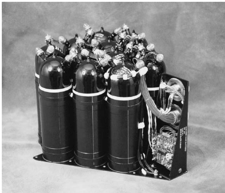
FIGURE 32.25 Mars Polar Lander 16-Ah CPV battery assembly.
