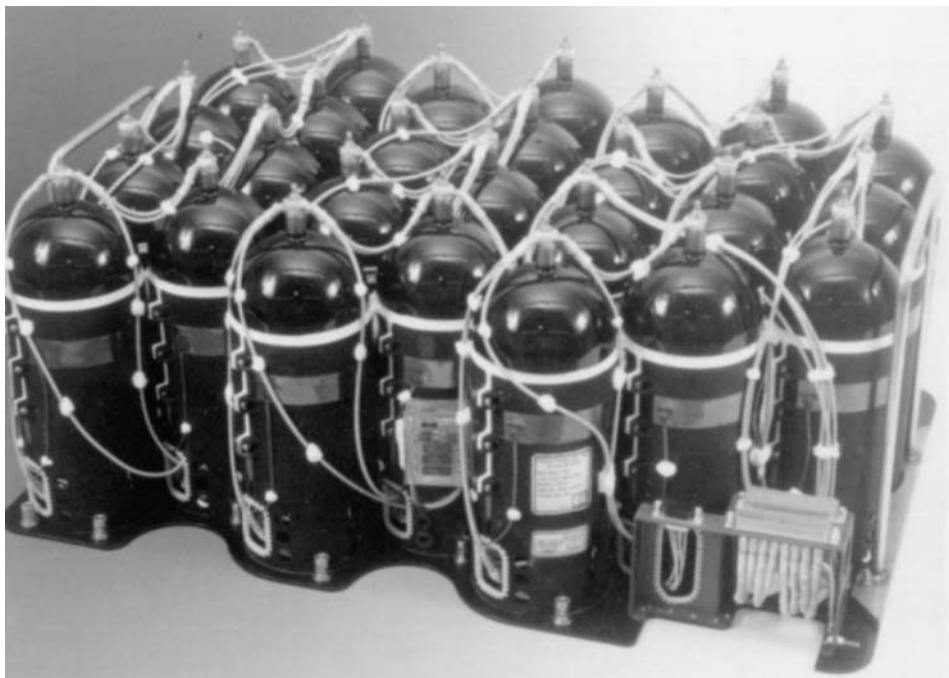
FIGURE 32.7 EUTELSAT II 58-Ah Ni-H 2 battery.
