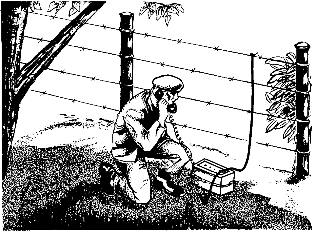
Figure 10-1. Expedient Ground return circuit.
