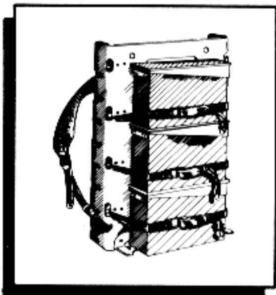
Figure 4-46. Load lashed with quick-release strap and clamp assemblies.
