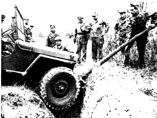
Figure 51. Pole used as a pry.
