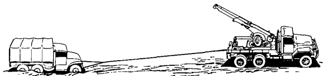
Figure 100. Recovering mired truck with a wrecker truck.
