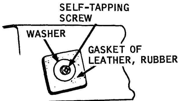
Figure 78. Pinhole-size leaks in fuel tanks.
