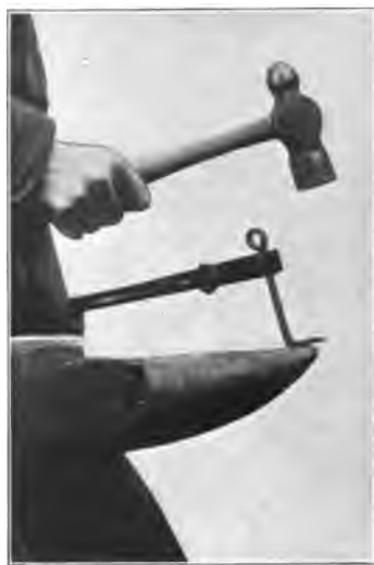
FIG. 18. BENDING THE POINT.
