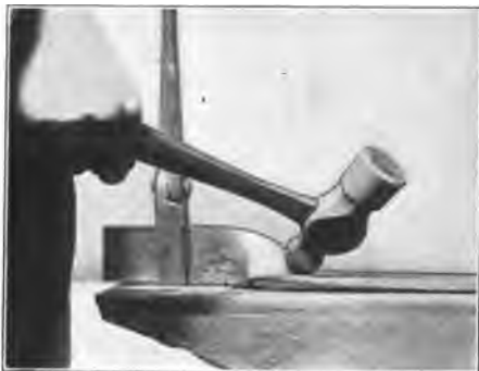
FIG. 35. HAMMERING DOWN THE CENTER.
