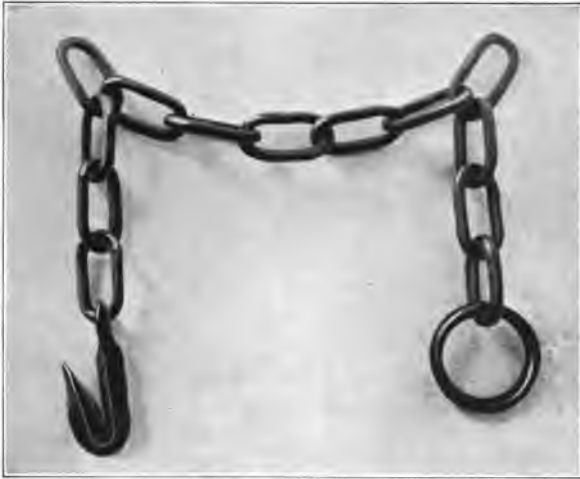
FIG. 41. CHAIN WITH RING AND GRAB HOOK.
