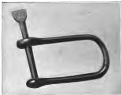
FIG. 45. LARGE WELDED CLEVIS.
