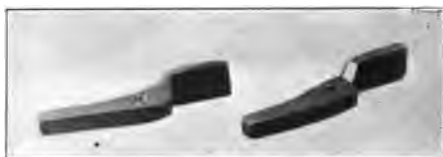
FIG. 55. TWO HEADS OF STRAIGHT LIP TONGS.
