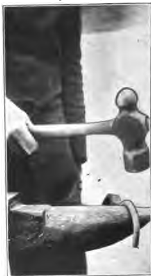
FIG. 13. BENDING OVER THE HORN OF THE ANVIL.
