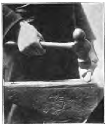
FIG. 42. FIRST STEP IN SHAPING A SCARF.
