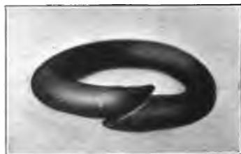
FIG. 37. SHOWING SCARFS ON LAP WELD OF RING.
