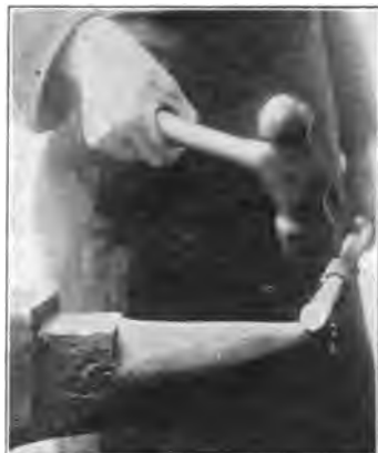
FIG. 43. BENDING POINT OF SCARF.
