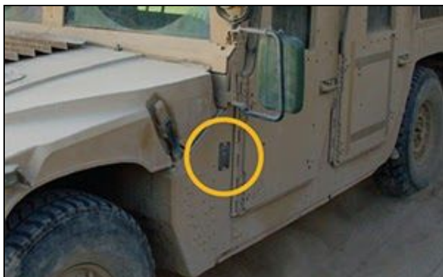
RFID tag mounted on a HMMWV.
