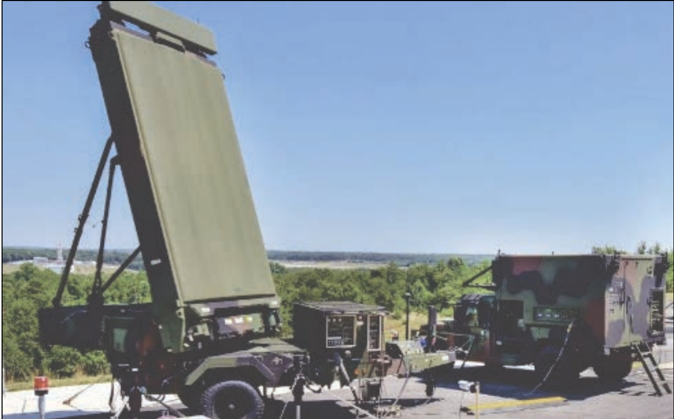
AN/TPS-80 G/ATOR (Ground / Air Task-Oriented Radar). Source: Northrop Grumman.
