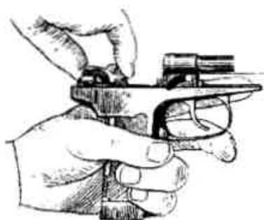
Picture 3.11 Removal of hammer from frame
