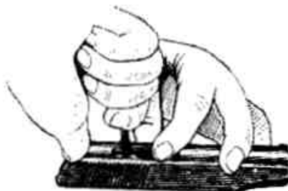
Picture 3.17 Insertion of the extractor into the slide
