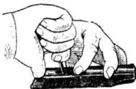
Picture 3.14 Removal of extractor from slide
