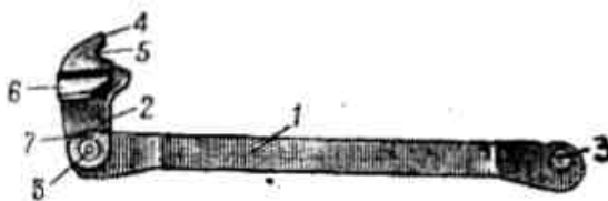
Picture 2.11 Trigger Bar with Disconnector
