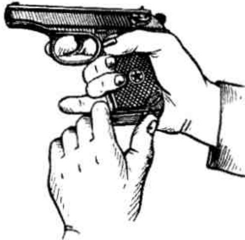
Picture 3.1 Removal of Magazine from the Frame
