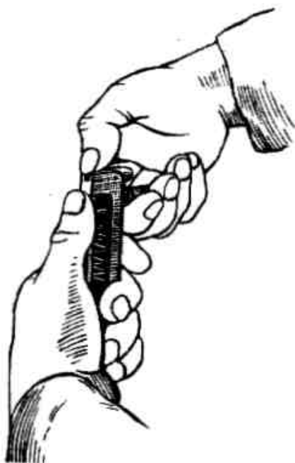
Picture 9.7 Removal of Cartridges from the Magazine
