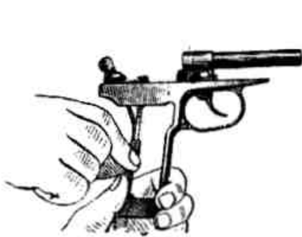
Picture 3.19 Insertion of the hammer into the frame
