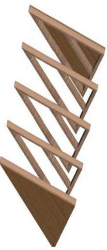
49) Rip a 8'-0" 2x6 (150x2400mm) plank as shown below. This will be a girder to stabilize the roof rafters. In areas of low snow loads, this step is not required. The girder will keep the rafters from warping under heavy loads.
