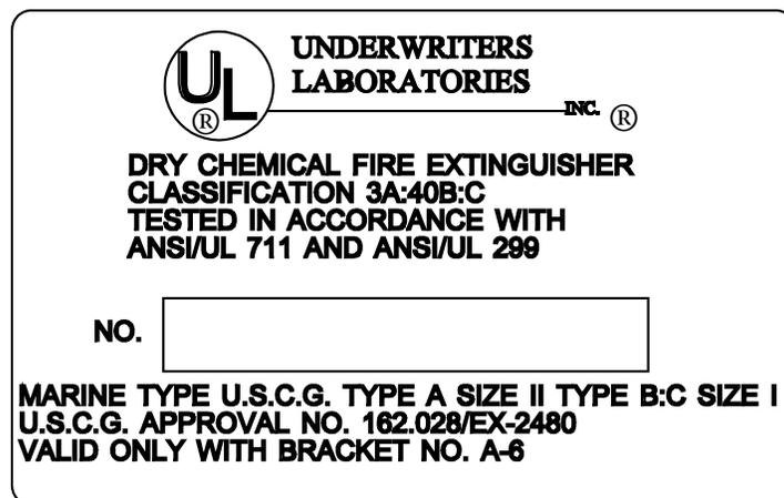
Sample manufacturer's label for a fire extinguisher, showing the Underwriters Laboratories symbol at the top, the type and classification of fire extinguisher, testing procedures used, and
