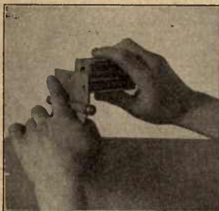
Fig. 137. Setting Gage for Depth of Gain
