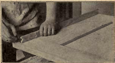
Fig. 134. Laying off Width
