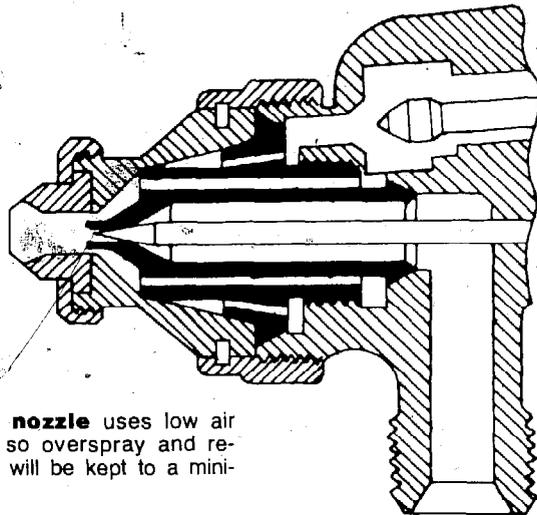
The internal-mix nozzle uses low air pressure and fluid, so overspray and rebounding of droplets will be kept to a minimum.
