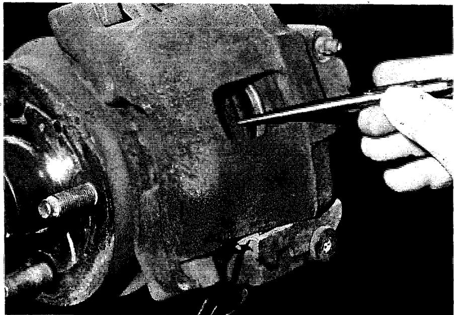
**Thickness of old vs new pads.** It doesn't happen very often, but a bad guy will tell you he installed new ones when actually he just left the old ones on. Check it out by removing a tire and looking through the caliper. It's easy to tell when new ones have been installed.
