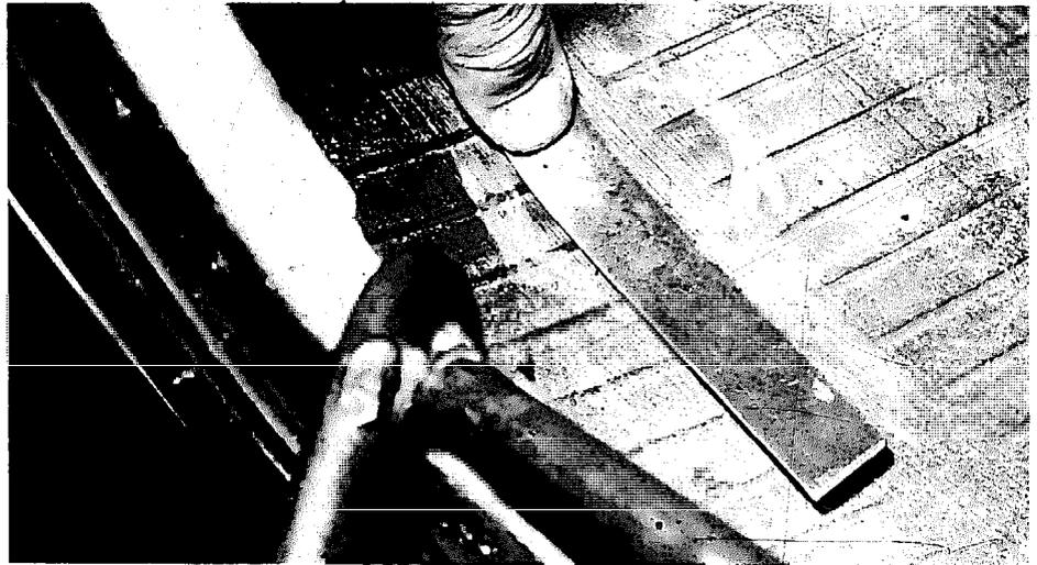
**STEP 4: Buff the area** lightly or scrape it with a wire brush to remove molded pattern on innerliner, but don't buff through the innerliner. Vacuum to remove dirt and rubber dust.
