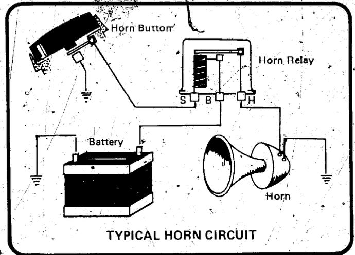
When horn button is depressed, electro-magnet inside relay pulls contact down to electrically connect horn with battery.
