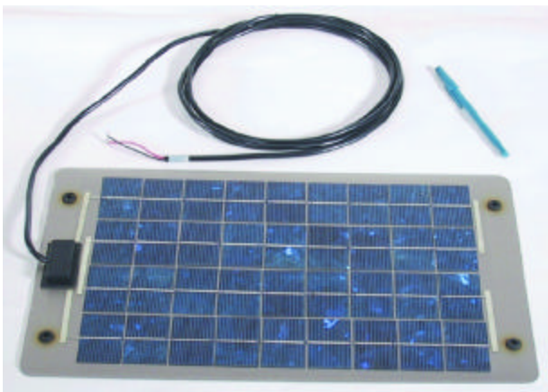
Inexpensive solar modules, 5 to 10 watts in size and 1 to 2 square feet in surface area, are adequate for maintaining a charge on an idle battery.
