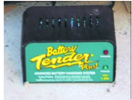
For equipment normally kept inside a shed out of the weather, your best charging solution is an electronic battery float type charger such as this 120-volt VAC battery float charger.
