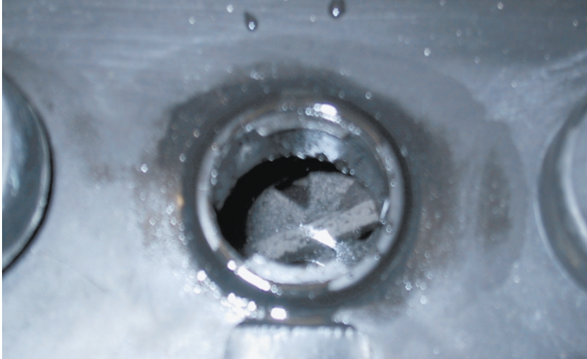
Looking into a lead-acid battery with the cap removed
