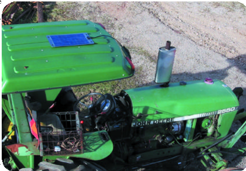
A small solar module, attached to the roof of this tractor, ensures that the starter will still turn over, even after a long period of idleness.
