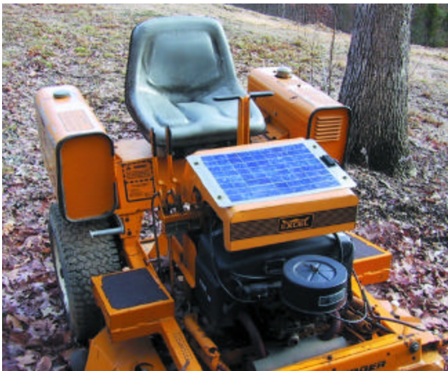
Even a small riding mower can benefit from the installation of a solar panel that ensures its battery is always ready.
