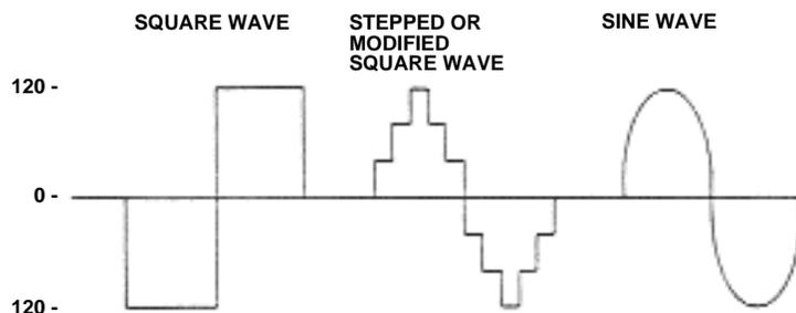
*The wave forms of various inverters from the most primitive simple square wave to pure sine wave. For most applications, the stepped wave will work well and reduce inverter costs.*
