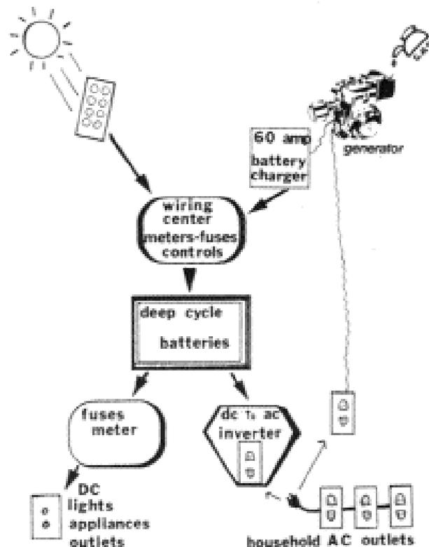
*Figure 1. Ingredients of a Home Solar Electric System.*
