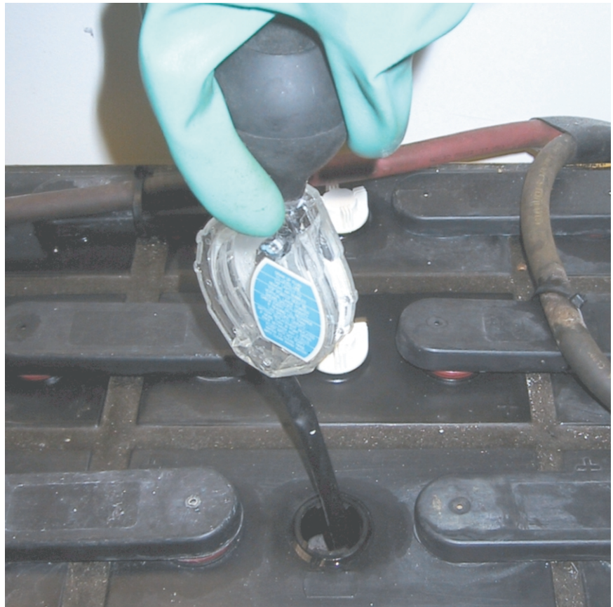
Checking battery electrolyte
