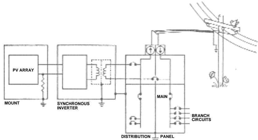
*The synchronous inverter interconnects the solar array to the home and the utility company. At the main distribution panel, power can flow in two directions.*
