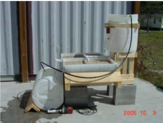
I make my aerator using a 3/4" npt to 1/2" barb fitting. I drill a 3/4" hole near the edge of the fish tank opening on the opposite end from the outlet.
