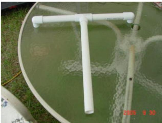
Next, using (3) 1/2" pvc ells, (2) 1-3/4" 1/2" pipe pieces, (1) 3" piece of 1/2" pipe and (1) 6" long piece of 1/2" pvc pipe assemble the adjustable siphon assembly as shown. These are slip fit and not glued.
