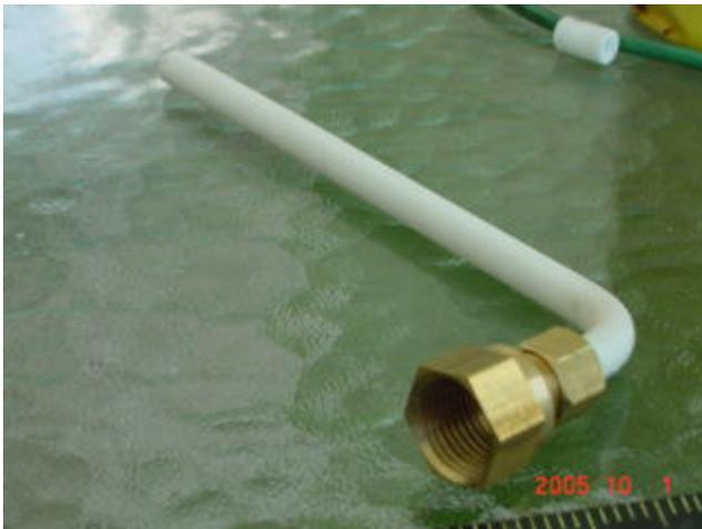
Disassemble the unit and remove the brass insert. Leaving it in place will restrict water flow through this tube.
