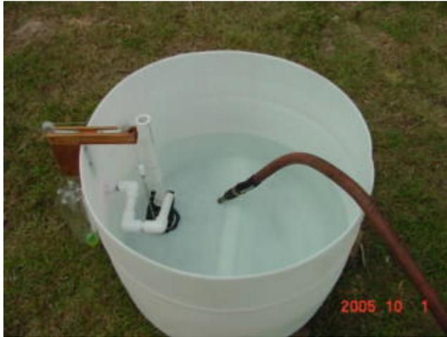
Watch as the water level approaches the top of the siphon. It should start filling the water bottle.
