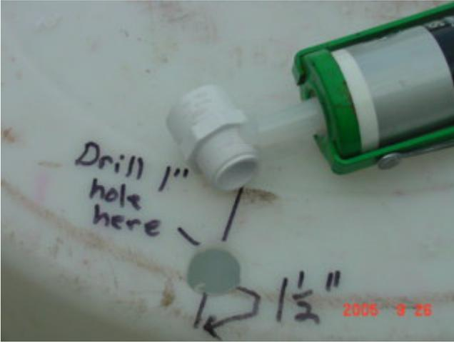
I prefer to lock the fitting on the inside with a conduit locknut to make the connection more secure. The threads sticking through to the inside can be used to secure a filter if desired.
