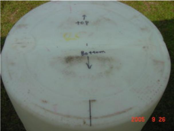
Remember the center mark on the mold line? Using a framing square make a line to the bottom of the tank and mark a point 1-1/2 " from the edge as shown.
