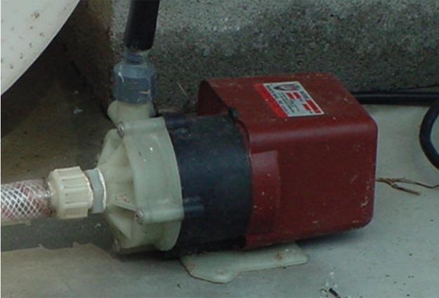
After hooking up the fish tank to the pump inlet I come out of the pump with the 1/2" black poly pipe and connect this tube to a "tee" with one side going to the raft tank and the other going to the fish tank hooked to a homemade aerator.
