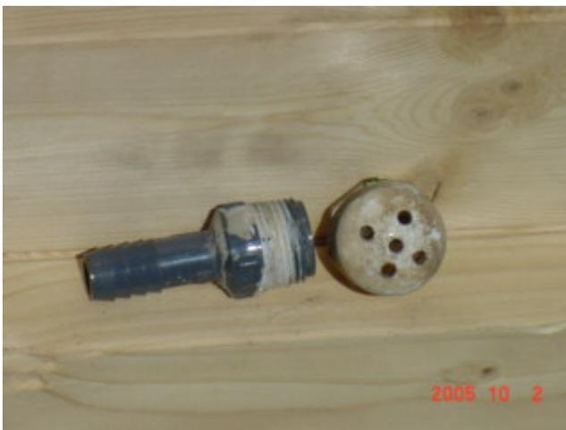
Fit the barb through from the inside with the barb sticking through to the outside. Slip the black poly tubing on here to capture the fitting in the edge of the fish tank (sometimes I have to warm up the tubing to make it easier to install).
