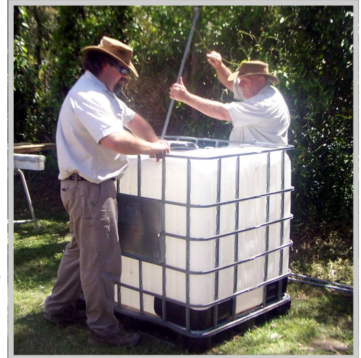
ABOVE:- Top braces/rails being removed from the IBC.
