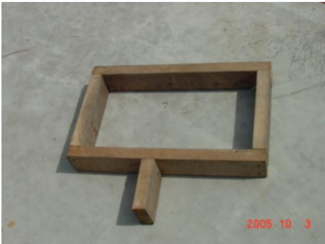
Notice the “leg” is offset from center to clear the roller block assembly
