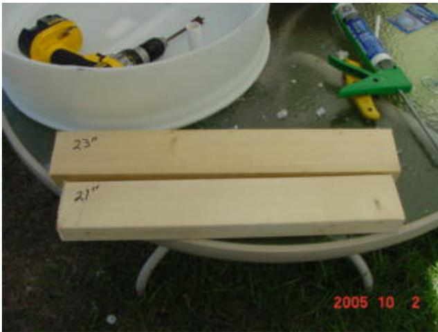
Using 3" deck screws make a "T" as shown. This is the spacer to set the raft tank on to the top of the flood tank.
