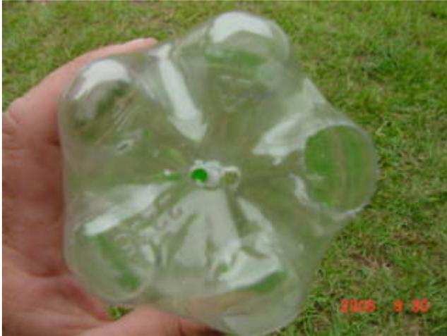
Flip over the bottle and drill a 5/32 hole in the cap. Don't worry too much about making a clean hole here. I wait until the unit is running and trim the hole as needed if the counterweight drains too slowly. If you mess this up just get another cap and try again until you get it right.
