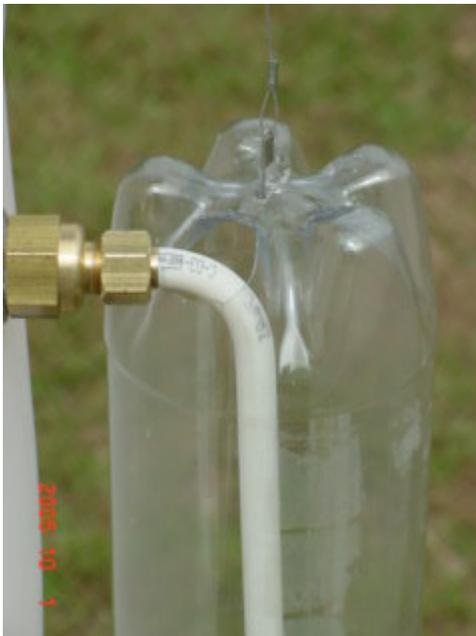
Install the adjustable siphon assembly to the male adapter as shown checking to see that the cable assembly clears the tubes through the full range of operation. There should be no binding in any part of the leader bottle movement. It should all move freely.
