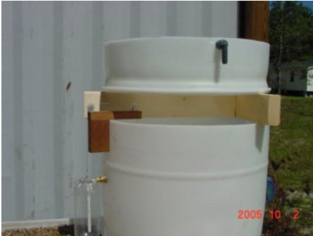
Another option that you could do instead of building a “tee” for the raft tank spacer you could make a rectangular bracket with a leg that would hold it on five points rather than three. This would help the tank not to sag as it will a little bit with the T-brace set-up. The sagging doesn’t seem to affect the operation of the unit. It just doesn’t look as good. The T-brace saves on lumber though.
