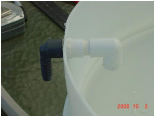
To adjust the flow from the pump one could pinch the 1/2" black tubing that runs from the pump to this fitting as needed. Adjusting flow to the tank will determine flood cycle times. Lower flow = longer time between floods. Higher flow = shorter time between floods. I usually use a 1/2" hose bib instead of the 1/2" male adapter, 1-3/4" section of pipe and 1/2" pvc ell to adjust the flow. An explanation of this is in the options section.
