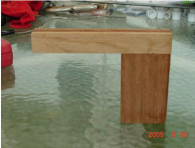
I cut a groove in the top for the rollers to sit in but it is not necessary as you can use the screw hole provided to mount the rollers directly on top and drill another hole and screw the rollers down securely. Cutting a groove eliminates the need for the second hole in each roller bracket.
