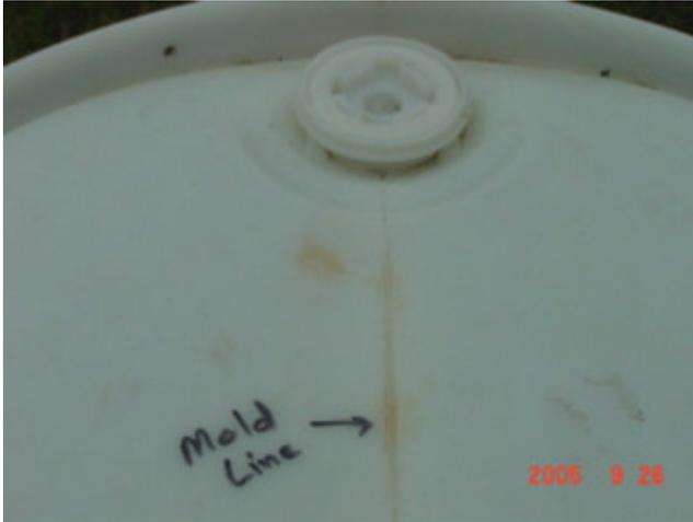
Find the middle of this line and using a framing square mark a point on the edge of the barrel 90deg. to the mold line on this mark.
