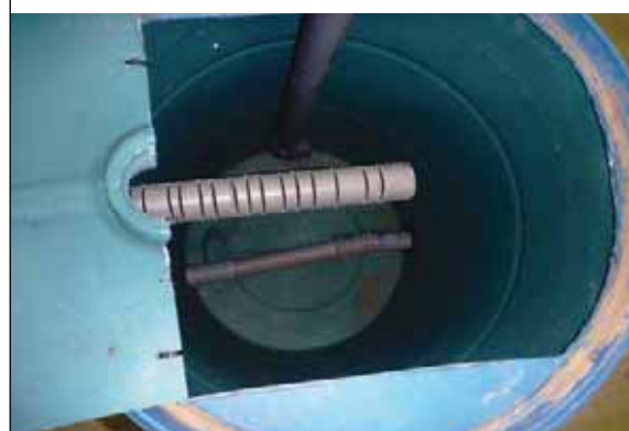
FIGURE 4.26 Picture of a mechanical solids separator
