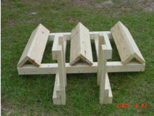
Now attach the 16" brace to the assembly as shown.
