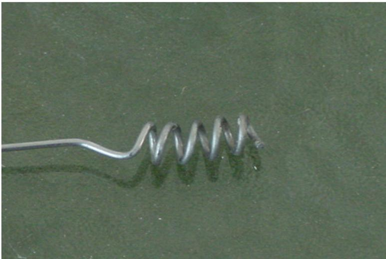
A couple of bends to make a simple crank and I have a tool that can fit inside the growbed drain tubes and grab the roots and rip them out to clear the drains.
