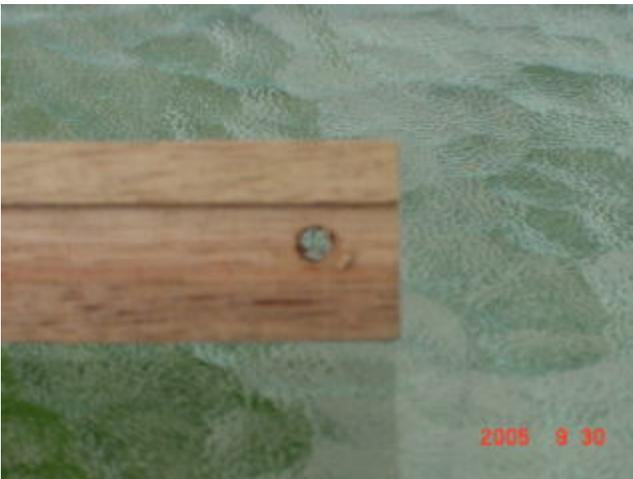
Screw the wood block pieces together using 1-5/8" deck screws as shown.
