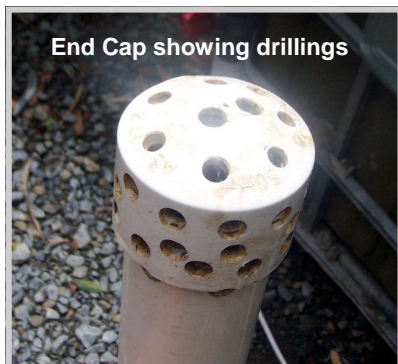
Above:- Fittings to bring water out from fish tank and on its way to the sump .
