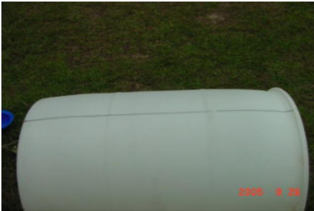
Measuring in from each end 6" draw a line 90 deg. to the centerline as shown in fig.4 on both sides of the line 6-1/2".
