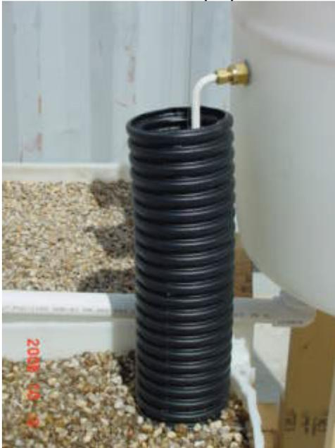
Mod with bottle in "down position". This will also help keep plant growth from fouling the operation of the floodvalve.
