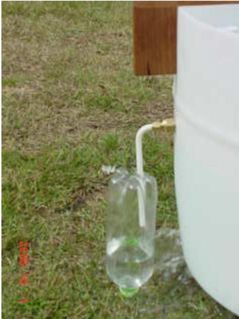
It is normal for the toilet valve to begin leaking a bit before it is fully pulled open. Continue filling the tank as it drains to mimic full time pump operation. When the water bottle empties it will allow the flapper to fall closed and seal off the tank for the next cycle. If the flapper didn't close properly you may need to add more washers to weigh it down. It should have just enough weight to close positively and no more! Too much weight will make the valve unnecessarily hard to open.
