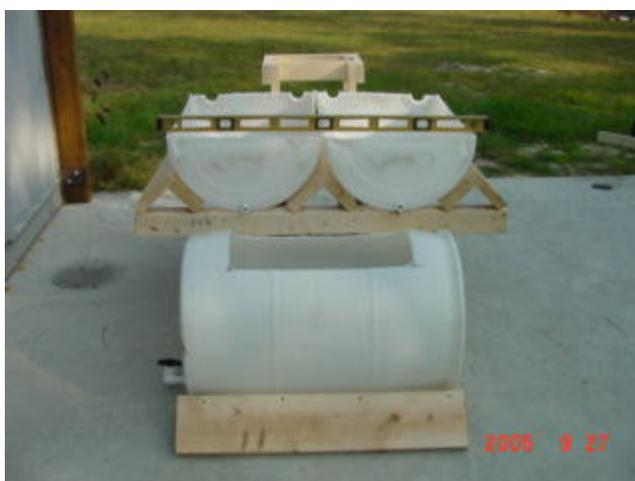
With the drain pipe halves in the bottom covering the suction tubes, hold down firmly while someone pours cleaned, washed pea gravel on top to hold the drain pipe halves down.
