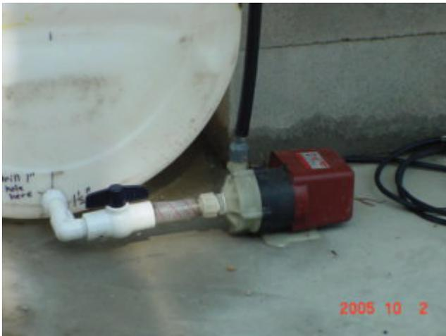
I would also advise using standard garden hose fittings as shown to make it a tool-less operation to clean out the inlet when needed.
