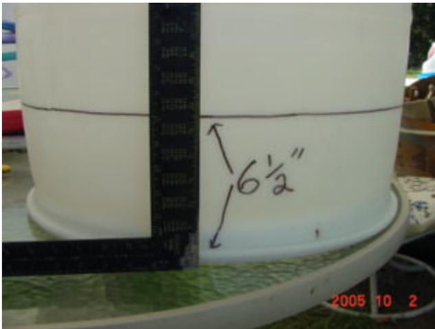
Cut the barrel here to make a shallow tank and drill a 1" hole about three inches in from the edge where the top is flat as shown. The actual distance is not all that critical as this is merely a standpipe to set the water level in the the tank.
