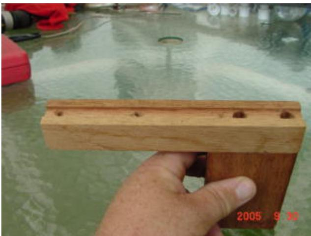
It would be helpful to install the steel leader at this time to help with the location of the rear roller. The leader is installed by threading the swivel end from the top down through the 5/32" hole at the rear as shown.
