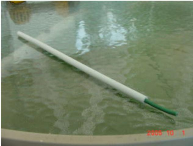
Gently heat a section 2" wide, back 1" from the end of the pipe until it is very soft and flexible. Form a 90 deg. bend around a piece of pipe and hold flat and in place until cool.
