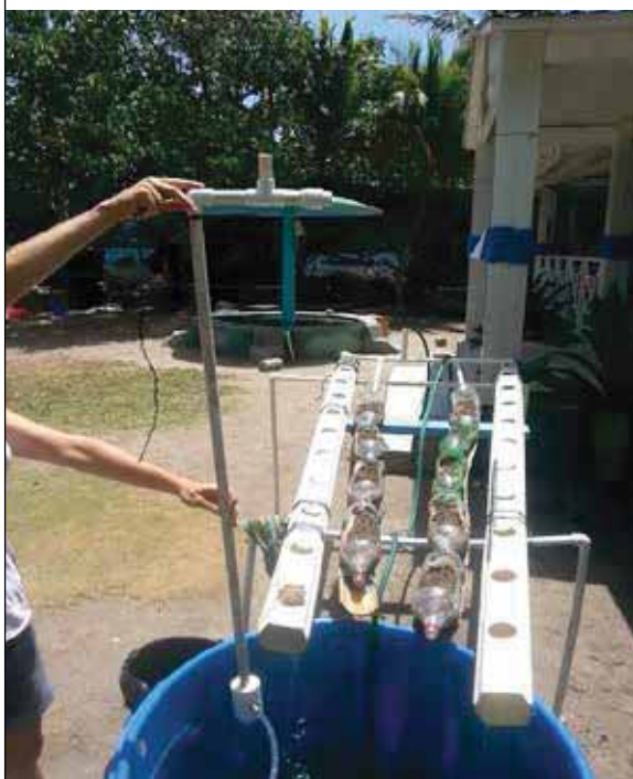
FIGURE 4.42 Simple water airlift
