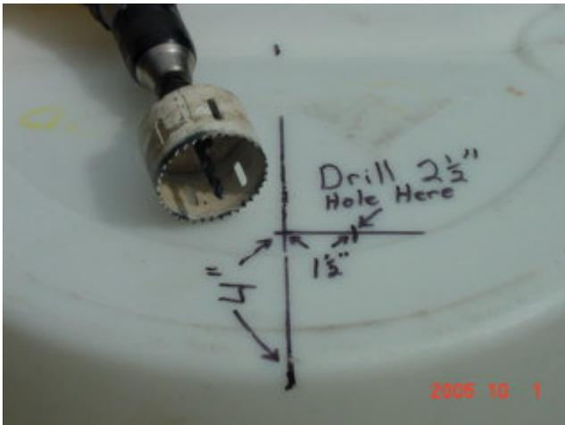
Using a 2-1/2" hole saw bore a hole centered on this mark. **Use extreme caution as hole saws can grab while cutting plastics. Be sure you have secure footing and control over your power tools during this operation!!! PLEASE BE CAREFUL!!!**
