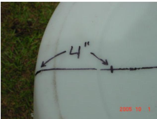
From this line using the framing square draw a perpendicular line 2" long from the 4" mark you just made.
