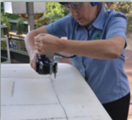
Use a straight edge to mark out your cut off point, once marked, use your angle grinder to carefully cut the top growbed section off the liner. Be sure to use a thin cutting blade for this.
