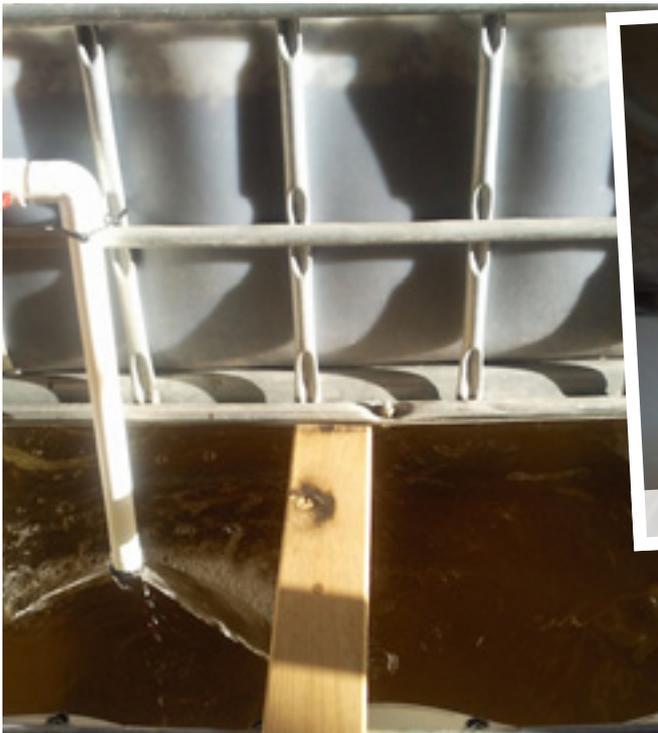
**Timber supports must be heavy duty to support the weight of heavy media beds**
