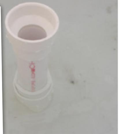
**The second type of siphon used in this system, an Affnan siphon**
