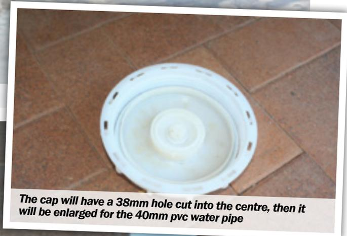
*The cap will have a 38mm hole cut into the centre, then it will be enlarged for the 40mm pvc water pipe*
