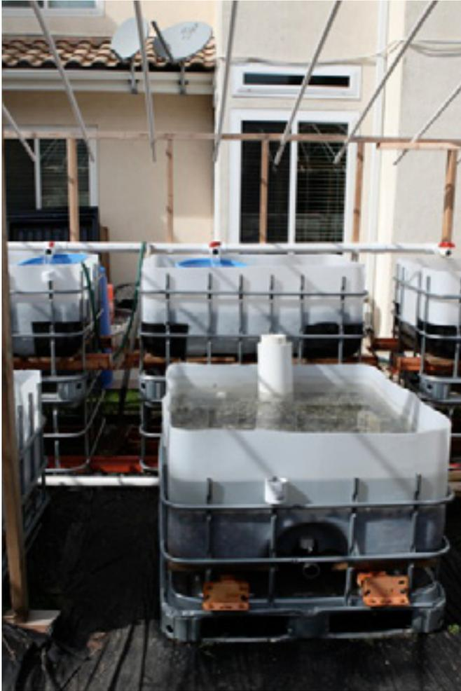
The fish tank with SLO (solids lift over flow)
