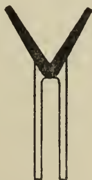
Showing piece split and forged to shape of jaw.
