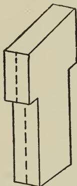
Showing how adjustable jaw is forged—dotted lines indicate where to split.
