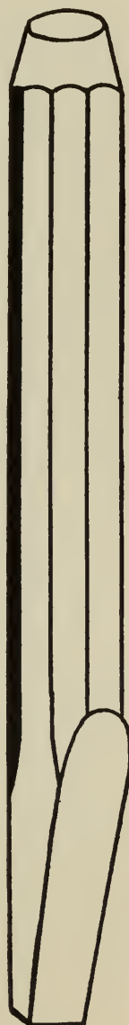
Fig. 57. The calking tool.
