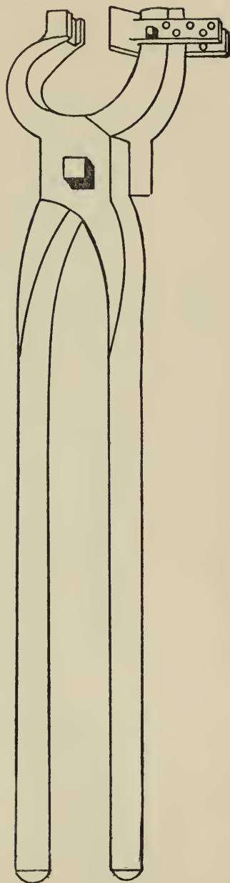
Fig. 4. Adjustable tongs regulated for holding largest size.
