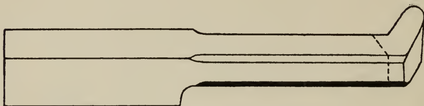
Fig. 42. The inside boring tool.
