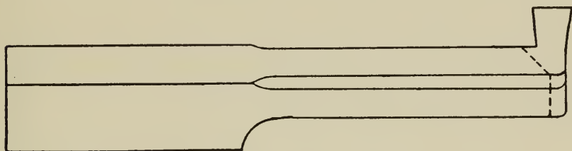
Fig. 44. The inside square thread tool.
