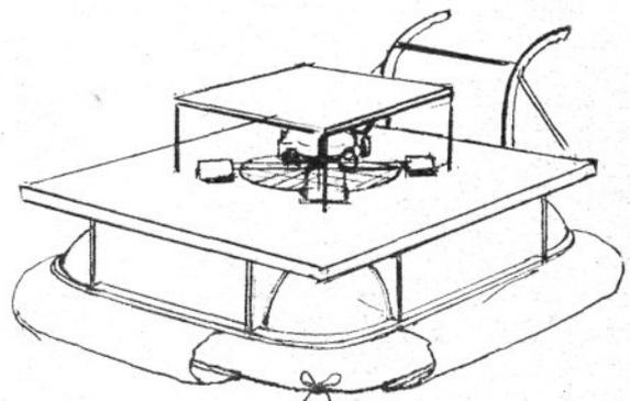
**AN OVERSIZE SKIRT** with a drawstring in the bottom edge may improve stability and performance as an air barrow over rough terrain.
