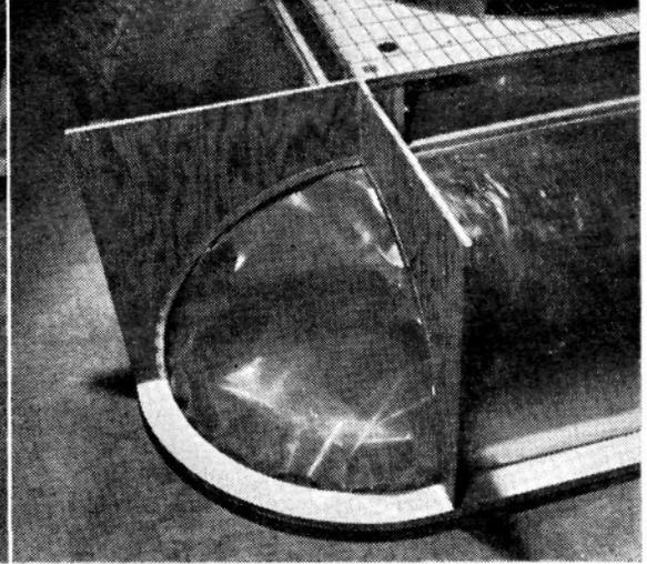
**ALUMINUM IS FASTENED** to inner curve of struts by bending a flange over flat against the plywood, and securing with stapling gun. Aluminum is slit every 1-1/2" to make a smooth bend.
