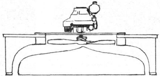
**CONVERSION TO AN ANNULAR JET** will be easy. According to theory, it should ride higher off the ground. I'll try a flat plywood bottom first, then tackle the problem of making a properly shaped core like this.
