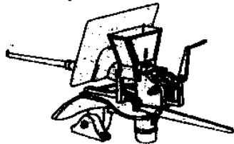
Agar "coffee mill" used steel cartridges, mid 19 th century
