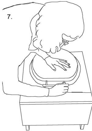
Mark holes for toilet seat attachment.
