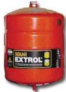
The expansion tank allows the fluid to safely expand by compressing the air in the chamber. The size of the expansion tank needed depends on the total volume of fluid, which is determined by the number and size of collectors, and the length and diameter of the pipes in the solar loop.
