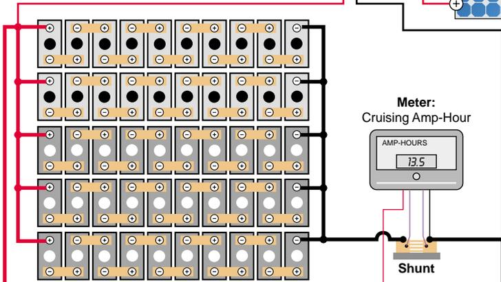
**Batteries:** Fifty nickel-iron cells wired in series strings of ten for 1,500 amp-hours at 12 VDC
