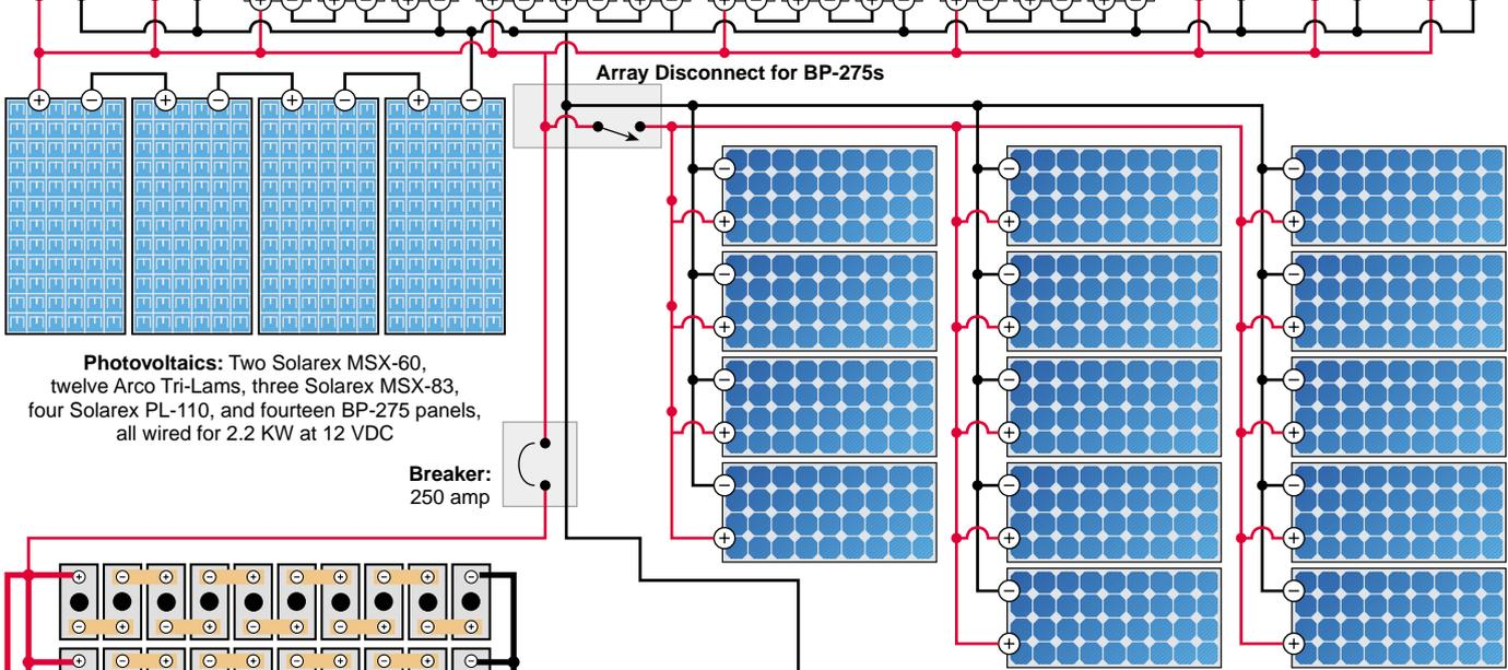
**Photovoltaics:** Two Solarex MSX-60, twelve Arco Tri-Lams, three Solarex MSX-83, four Solarex PL-110, and fourteen BP-275 panels, all wired for 2.2 KW at 12 VDC
