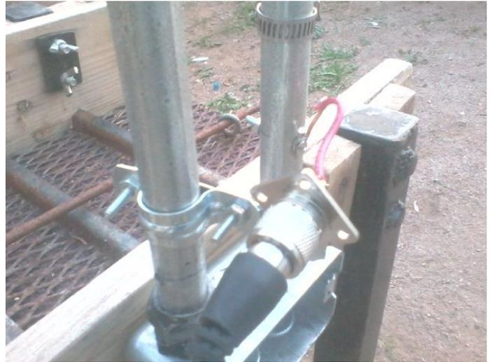
**Dave, K7AV:** My version uses the larger electrical box which allows using U-bolts to attach it to a mast, as shown below. I'm very happy with the results.
