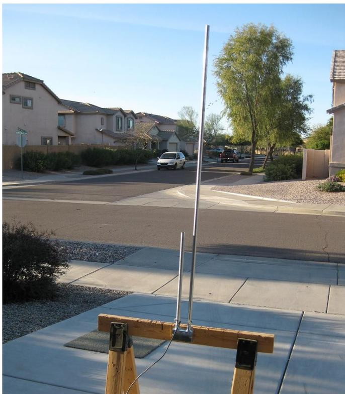
"Queen Creek Easy J" is presented as the electrician's delight. It requires almost no tools to assemble. You need one 57 inch long and one 19 inch long piece of 1/2 inch conduit, one steel duplex outlet box and two conduit adapters.
