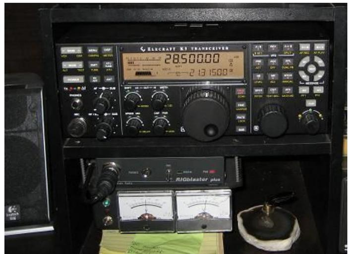
emergency 12 volt battery charger at the operating position. Just below the rig blaster is the dual meter display that shows the voltage of both the batteries and the TGE booster output.
