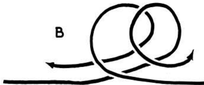
B. Turn both ends into eyes on the opposite sides, alongside the other standing parts.
