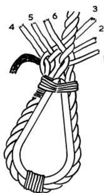
H At the other side, tuck the remaining strands in turn, each under one.
