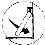
FIREBRICKS ARE TO BE INSTALLED BEFORE FIRING STOVE.
