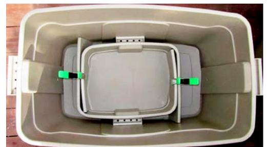
**Step 9:** Place the two sections into the outer container and arrange so that the two sections align to fit squarely against both sidewalls. Use two spring clamps to hold the sections in place.
