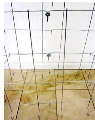
**Step 3:** Place **one** 1/8 inch Wire Rope Clip as shown over the top endpoint pair (only) and secure tightly. Note: you will attach the wire rope clips to all endpoint pairs after the cage has been mounted on the EarthTainer. This provides additional flexibility when wrapping the cage legs around the rim of the container.
