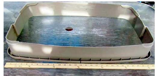
**Step 7:** Rotate the piece 180 degrees on the work surface, then find the center rib at the 14 inch mark, and repeat the 2 vertical lines at the center rib, and again 3 inches to the right (at the 17 inch mark).
