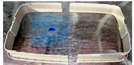
**Step 8:** Invert, then arrange the two sections interleaved with each other placing the shorter sections to the inside, and the longer sections wrapping around the outside. The objective is to get a rectangular, symmetrical assembly.
