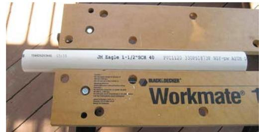
Approximately 1" up from the bottom, drill two 3/8" diameter holes through both sides of the pipe. Move up another inch and repeat drilling another 2 holes.
