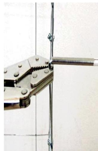
Consistency is most important in making the 3 bends. The goal is to get each 90 degree bend such that the mark falls on the inner or outer radius. The tighter the fit of the Tube to the cage, the sharper the bend that can be made at each mark.
