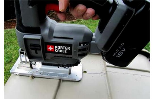
If you do not have a power jig-saw, you can use a sturdy pair of kitchen scissors or tin snips to manually cut the container along the scribe mark (this will require good hand strength).
