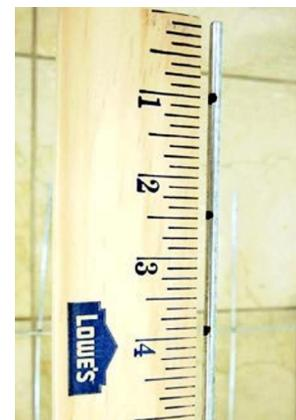
**Step 5:** Use a 1/4" O.D. diameter Stainless Steel Tube (see recommended Tools in the Appendix) along with heavy-duty vise-grip locking pliers to make each of the three 90 degree bends. Always lock the pliers on the opposite side of the bend. This will give you maximum leverage and will permit a crisp sharp bend at the marker points.
