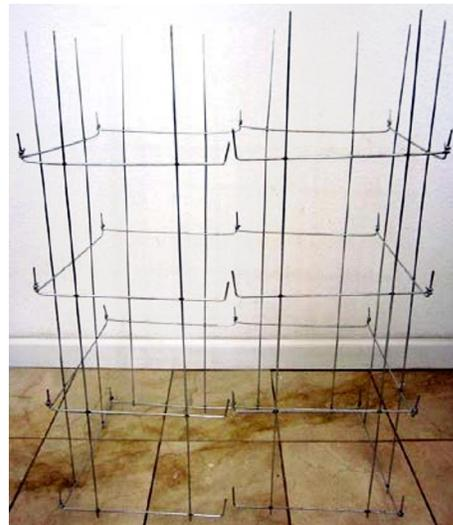
**Step 2:** Using a Nut Driver, straighten the 8 endpoints so they are in vertical alignment.
