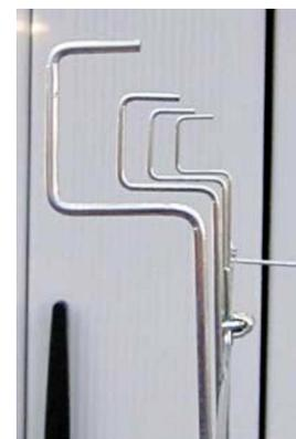
**Step 8:** The extension cage can be attached to the base cage either before the cage system is attached to the EarthTainer, or can be mated to the base cage as needed later in the Season (recommended). For immediate attachment to the base cage, invert the cage and bend all of the legs at a very slight inward angle.
