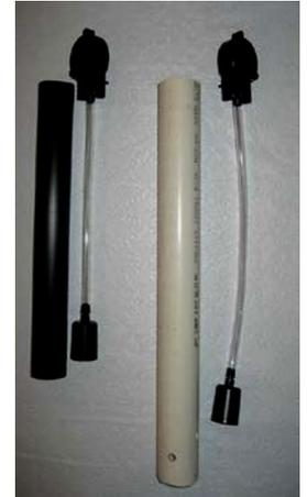
Reconnect a 13" section of new hose. This is common Ice Maker hose found at Home Depot or Lowes in 10 or 20 ft. sections. Reinstall the filler tube and insert the lengthened AWS unit into the EarthTainer. Connect the Pressure Regulator and tubing as per the supplied instructions.
