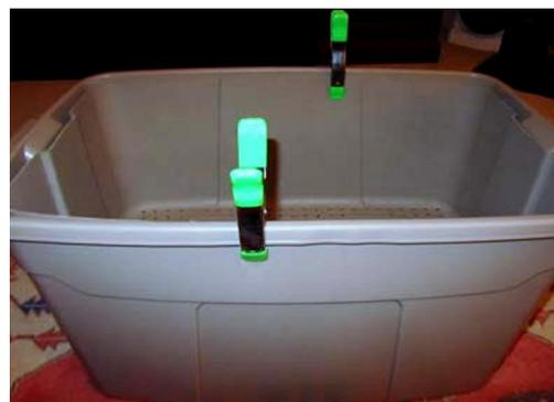
Locate the center rib (#7) and make a mark down 5-1/2 inches from the top of the container. Using a 1/4 inch drill-bit, drill through both the outer container as well as the Aeration Bench. Be mindful of where your hands are at all times!!
