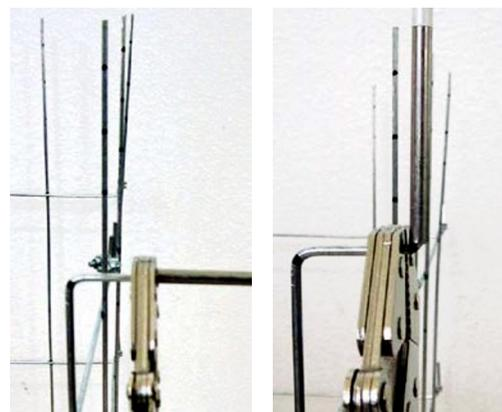
**Step 6:** Unclamp the pliers from the first bend, and now locking them at the next bend at the 2-1/2 inch marking, 1/16 inch to the inside of the mark, facing upward. Make this second 90 degree bend up in the vertical direction.
