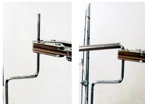
With the Tube sleeve, bend the final section 90 degrees inward.
