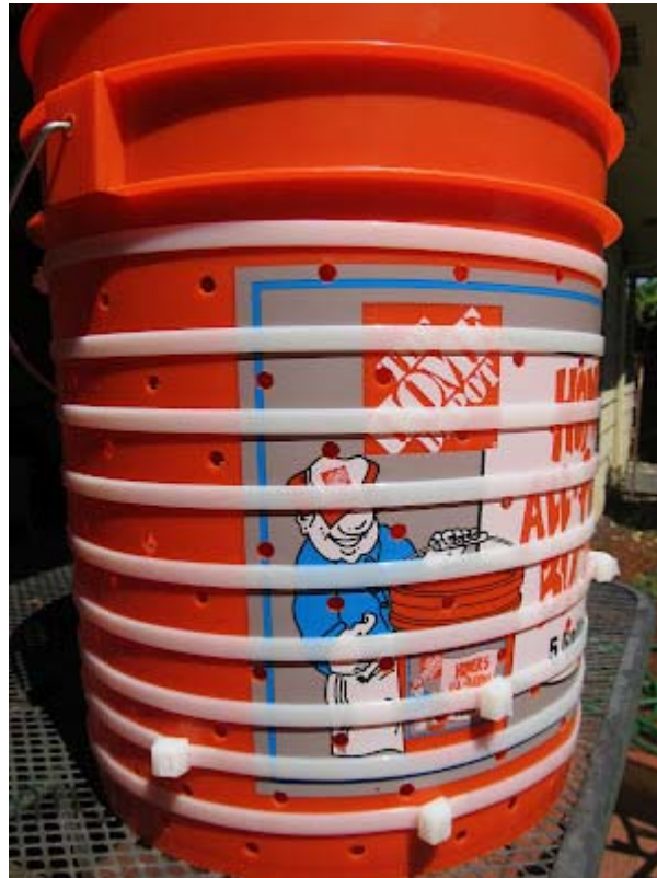
DIY apple cider press basket made from Home Depot bucket.
