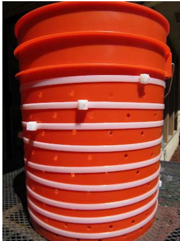
Apple Cider Press Basket With Zipties For Strength.
