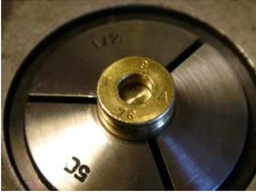
Then you need to make a center mark on the flat bottom of the pocket for the small thru flash hole. A regular #3 drill will do fine if you are careful to bring it down without hitting the sides hard.
