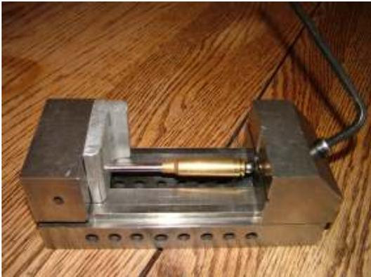
I marked the brass with a felt tip so you could see the shiny area where the metal was moved. This will be a ridge smaller than the diameter needed.
