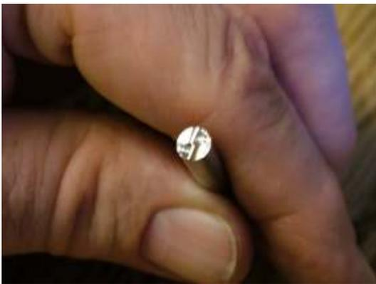
As you can see, the tool cut the anvil out nicely without more than burnishing the pocket wall.
