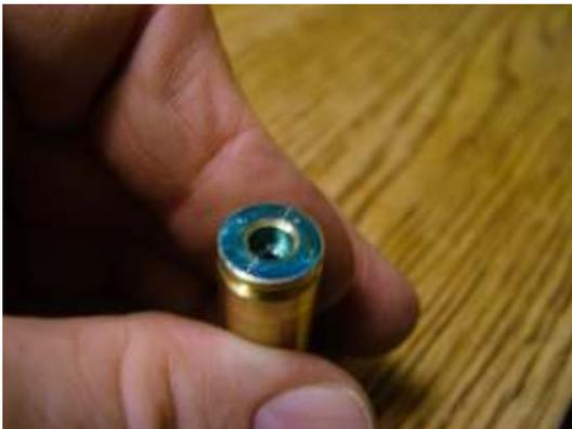
We need a rather exact fit to press a primer in. I ran a .209 gage pin into the pocket to counter swag the hole. Just to make sure I also ran a .209 reamer in too. It accepted a Boxer primer with a good fit.
